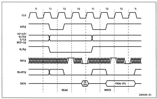
Figure 7.8. Basic 3-3 Bus Cycle
