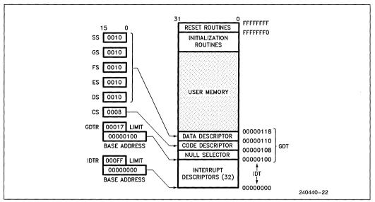
Figure 4.17. Simple Protected System
