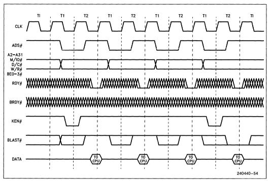
Figure 7.11. Non-Burst, Cacheable Cycles
