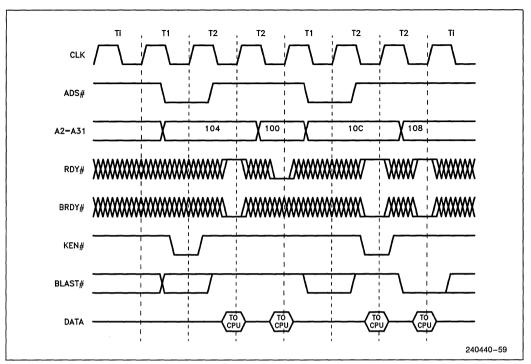
Figure 7.16. Interrupted Burst Cycle
