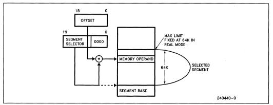
Figure 3.1. Real Address Mode Addressing
