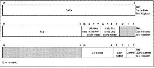
Figure 8.4. Cache Test Registers
