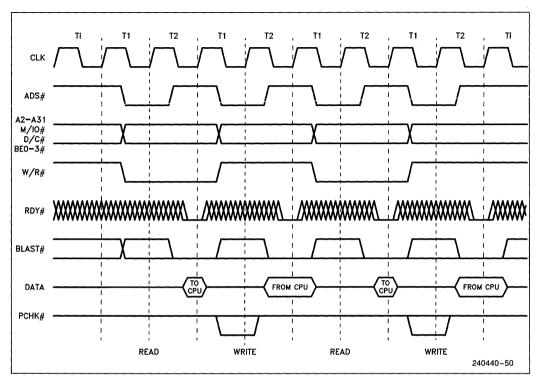
Figure 7.7. Basic 2-2 Bus Cycle
