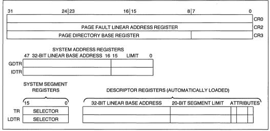
Figure 2.4. System Level Registers
