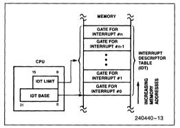
Figure 4.4. Interrupt Descriptor Table Register Use
