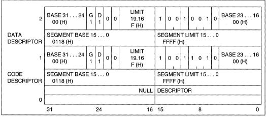
Figure 4.18. GDT Descriptors for Simple System
