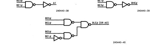
Figure 7.5. Logic to Generate A1, BHE# and BLE# for 16-Bit Busses
