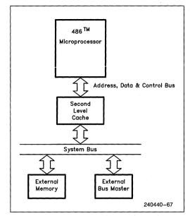
Figure 7.24. System with Second Level Cache
