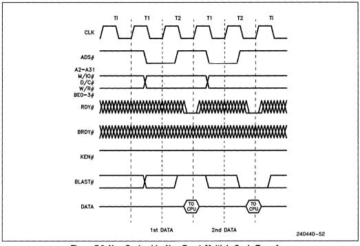
Figure 7.9. Non-Cacheable, Non-Burst, Multiple Cycle Transfers
