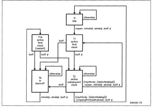
Figure 7.30. Bus State Diagram
