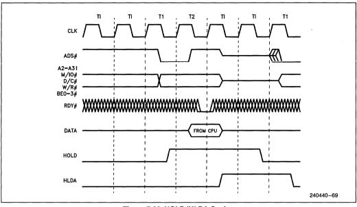
Figure 7.26. HOLD/HLDA Cycles
