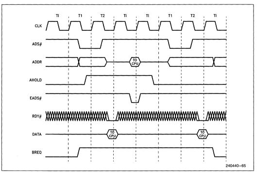
Figure 7.22. Fast Internal Cache Invalidation Cycle
