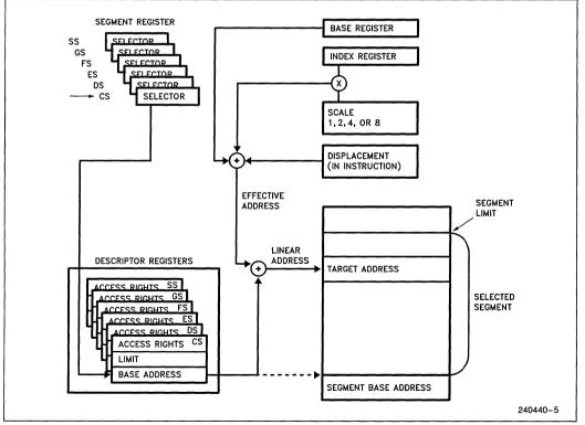
Figure 2.17. Addressing Mode Calculations
