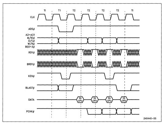
Figure 7.12. Burst Cacheable Cycle
