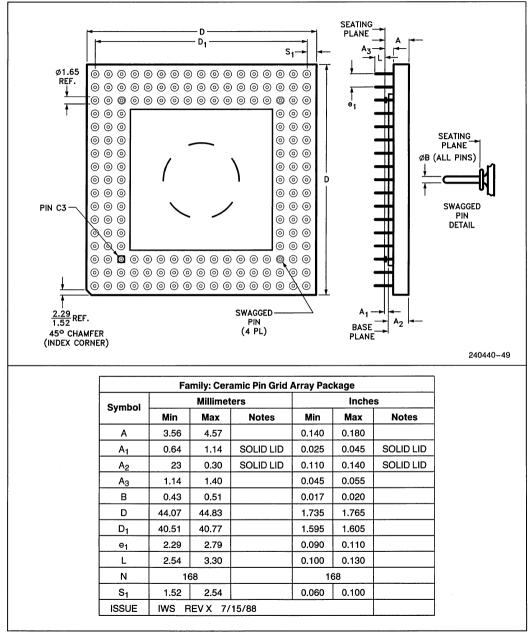
Figure 13.1. 168 Lead Ceramic PGA Package Dimensions
