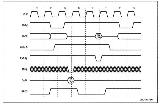
Figure 7.23. Typical Internal Cache Invalidation Cycle
