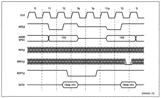
Figure 7.29. Restarted Write Cycle
