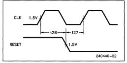
Figure 6.3 Reset Waveform
