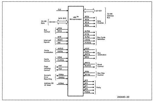
Figure 6.1. Functional Signal Groupings
