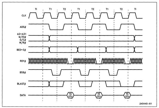
Figure 7.18. 8-Bit Bus Size Cycle
