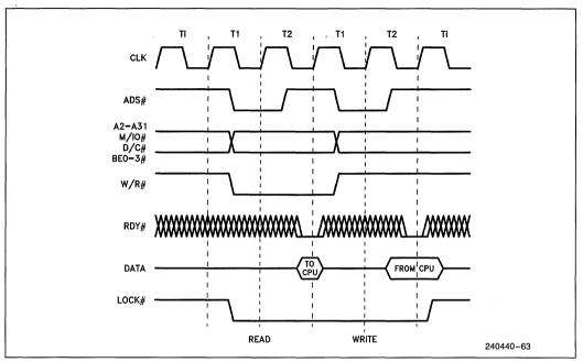
Figure 7.20. Locked Bus Cycle
