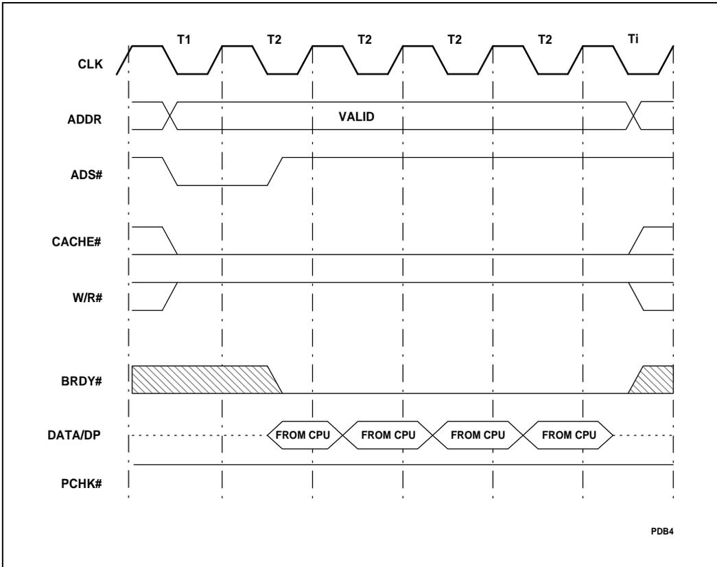
**Figure 6-10. Basic Burst Write Cycle**
