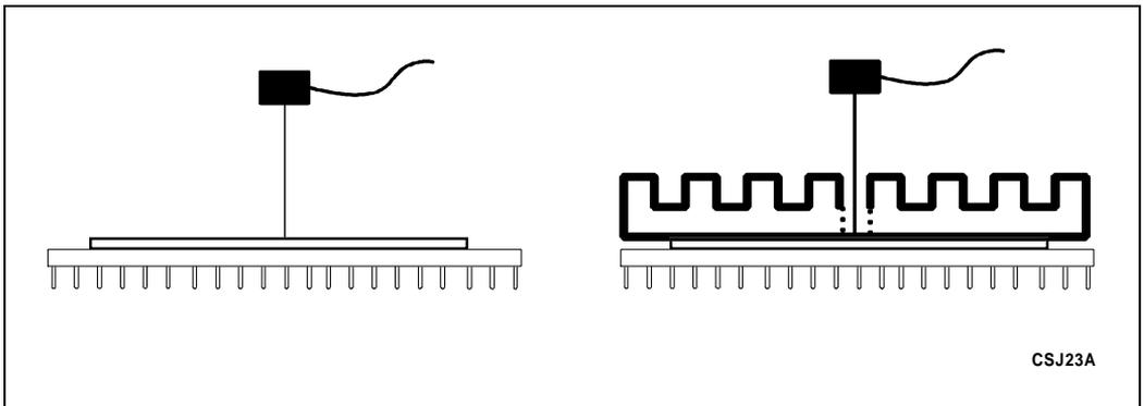
**Figure 10-1. Technique for Measuring  $T_{case}$ \***
