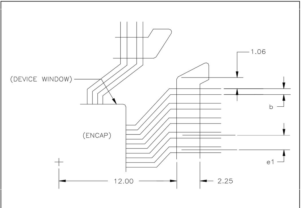
Figure 34-6. Outer Lead Bond (OLB) Window Detail
