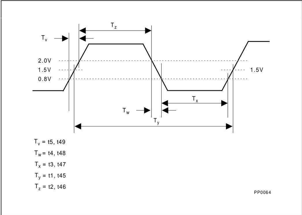
Figure 7-1. Clock Waveform
