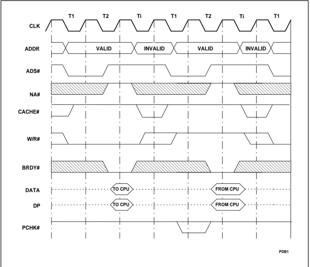
Figure 6-6. Non-Pipelined Read and Write
