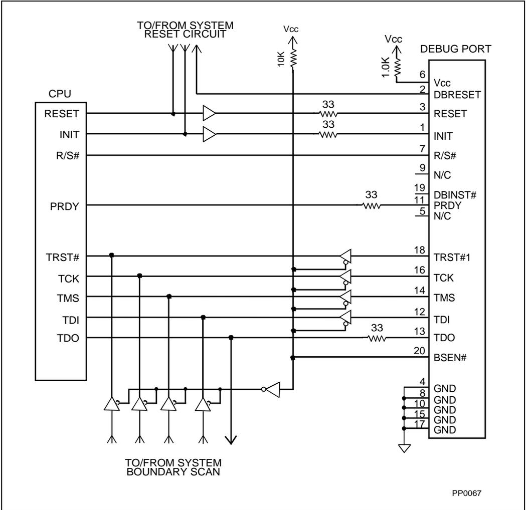
Figure 31-3. Single CPU — Boundary Scan Used
