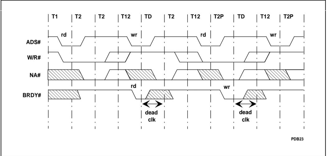
Figure 6-31. Bus Cycles with TD Dead Clock
