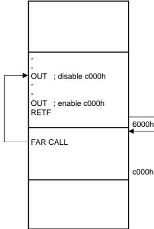
The branch prediction mechanism of the Pentium processor, however, predicts that the RETF instruction is going to transfer control to the segment at address c000h and performs a prefetch from that address prior to the OUT instruction that re-enables that memory address. The result is that no BRDY is returned for that prefetch cycle and the system hangs.
