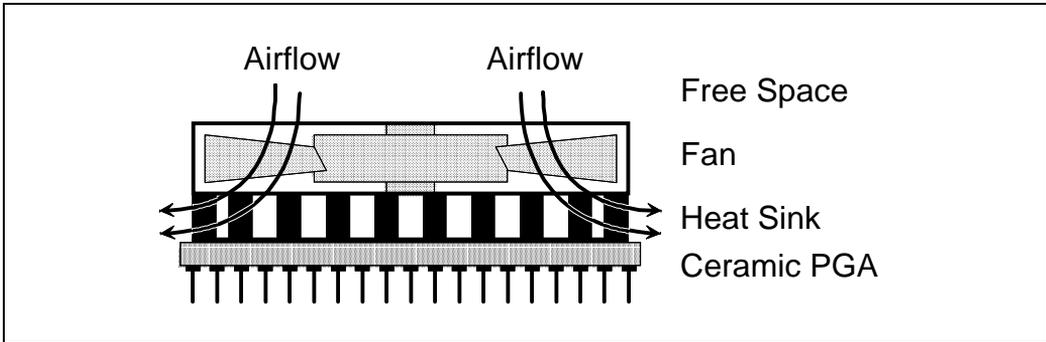
**Figure 16-8. Fan/Heatsink Example**
