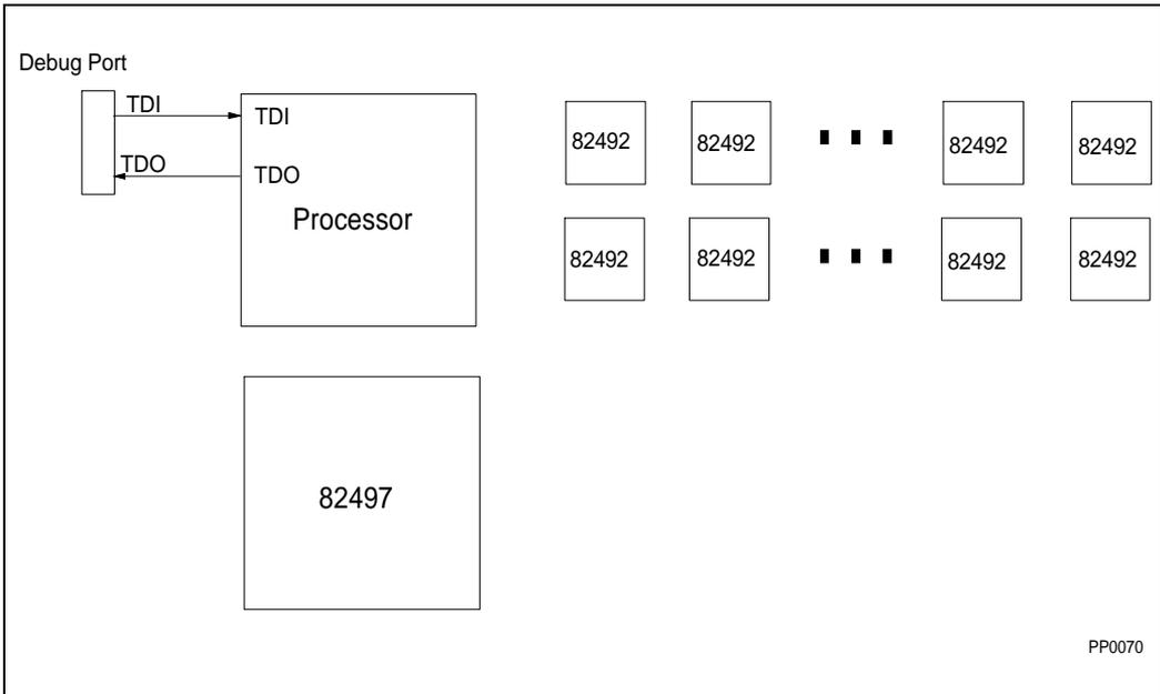
Figure 31-6. Example of CPU Only in Scan Chain
