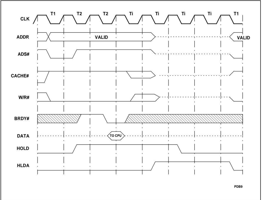
Figure 6-15. HOLD/HLDA Cycles
