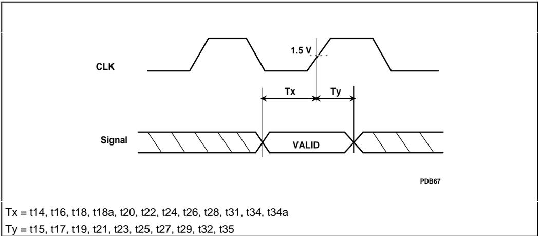
Figure 7-4. Setup and Hold Timings
