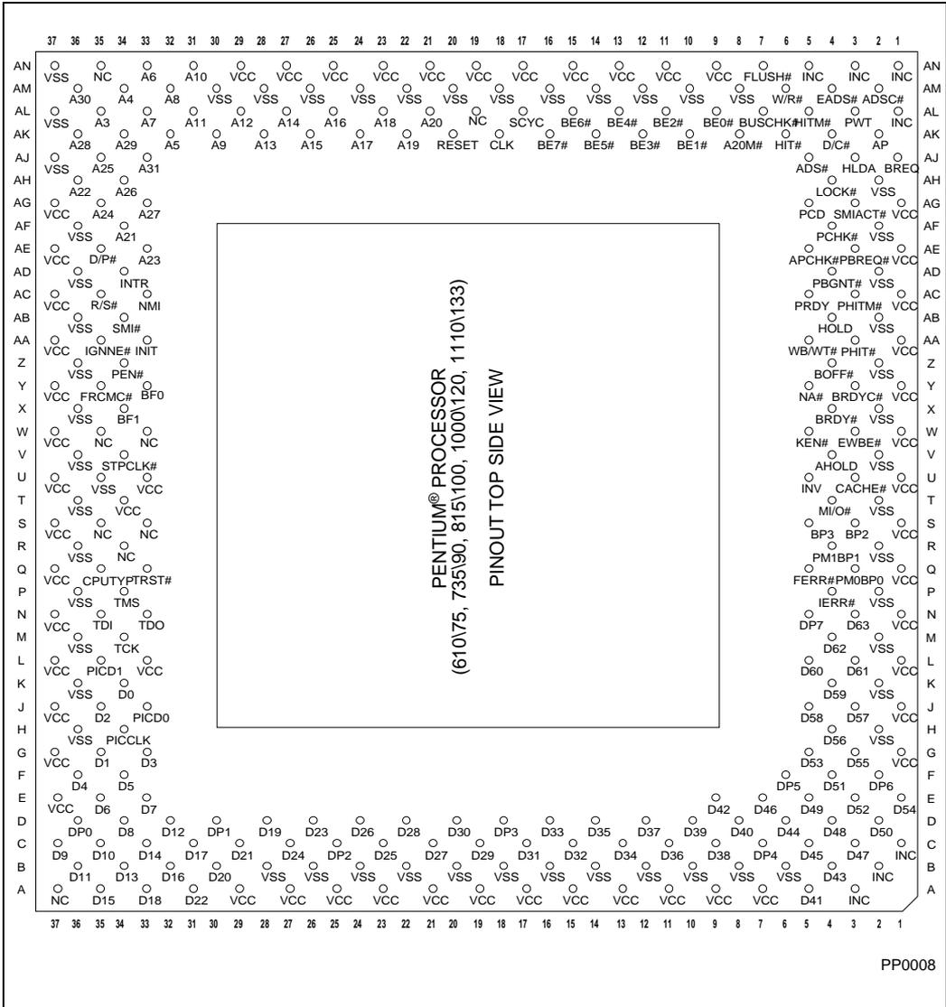
Figure 17-1. Pentium® Processor (610\75, 735\90, 815\100, 1000\120, 1110\133) Pinout — Top Side View
