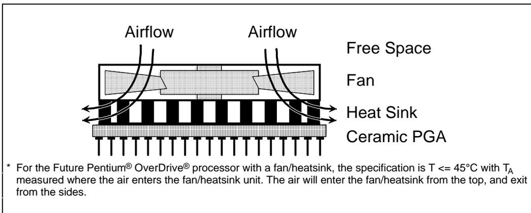
Figure 32-4. Thermal and Physical Space Requirements
