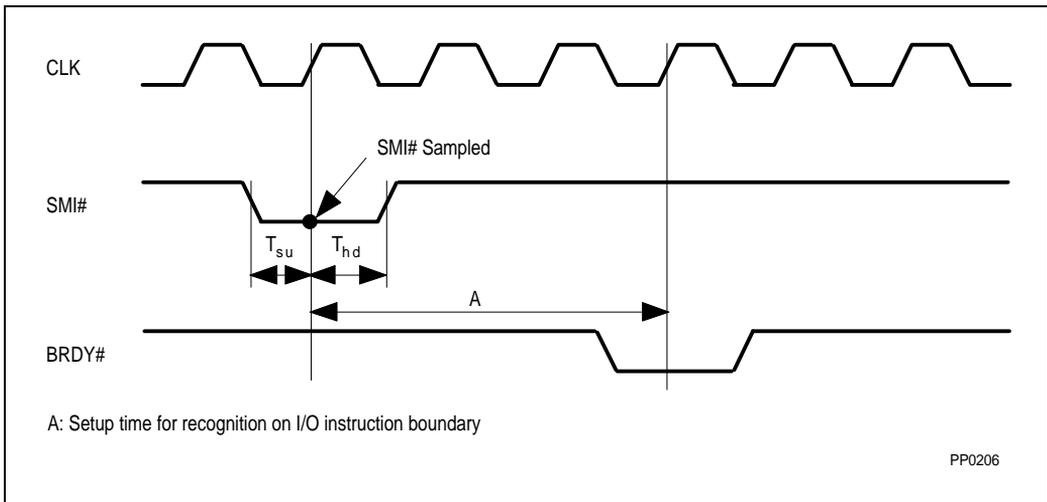
Figure 30-1. SMI# Timing for Servicing an I/O Trap
