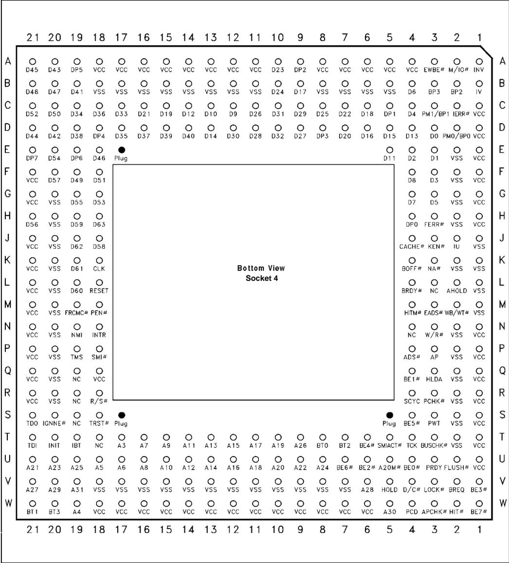
Figure 16-4. OverDrive® Processor Pinout (Bottom View)
