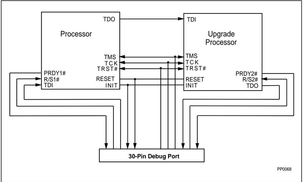
Figure 31-10. Shared Pins for Dual Processor Adapter
