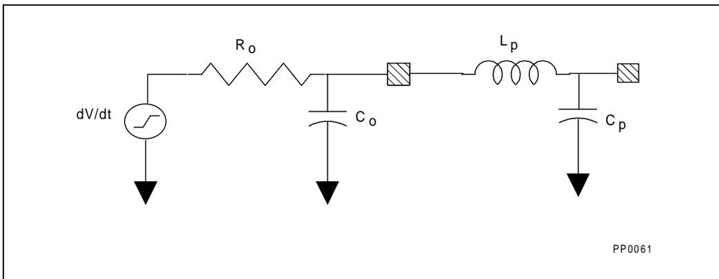
**Figure 24-3. First Order Output Buffer Model**
