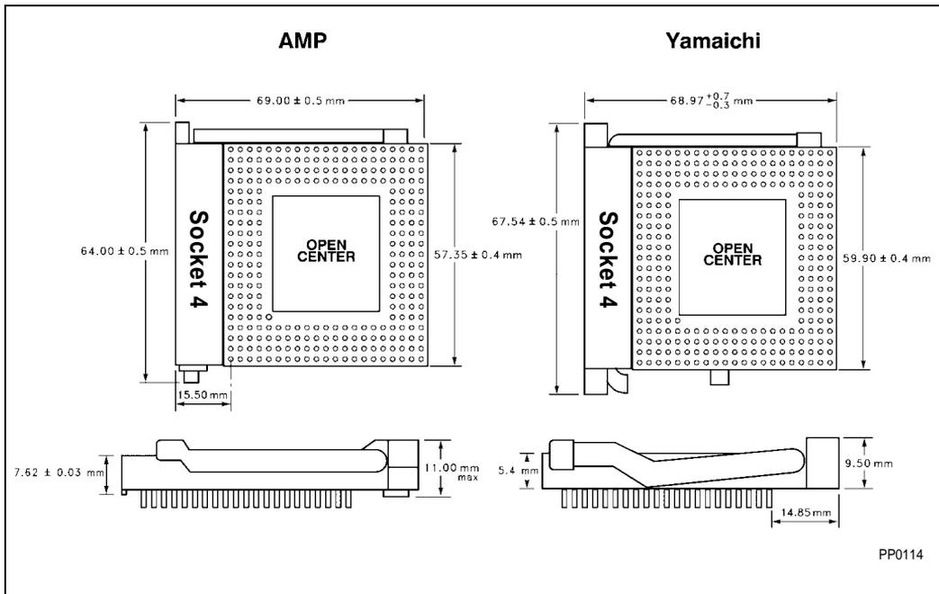
**Figure 16-1. Socket 4 Footprint Dimensions**
