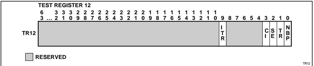
Figure 33-4. Test Register TR12
