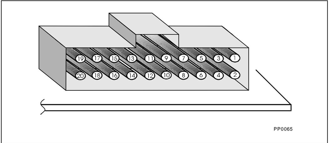
Figure 31-1. Debug Port Connector
