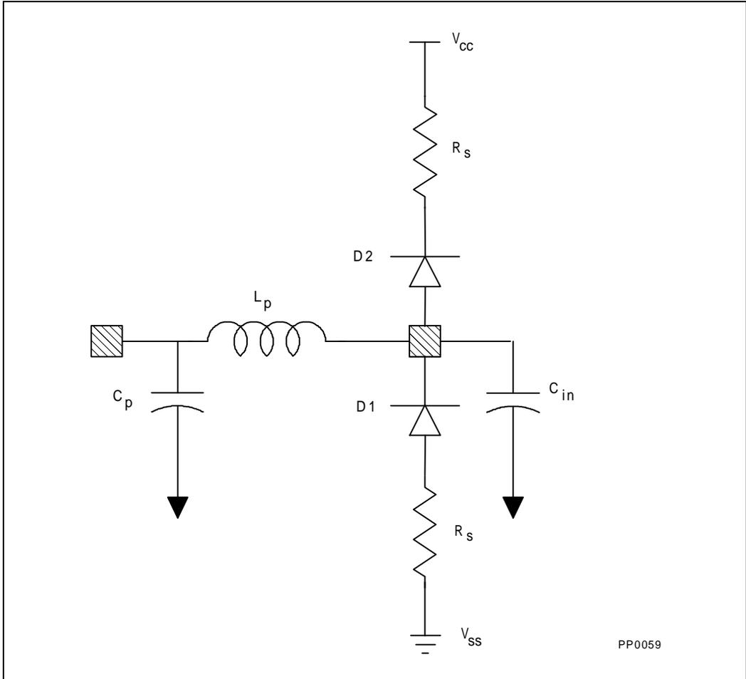
Figure 24-1. Input Buffer Model, Except Special Group
