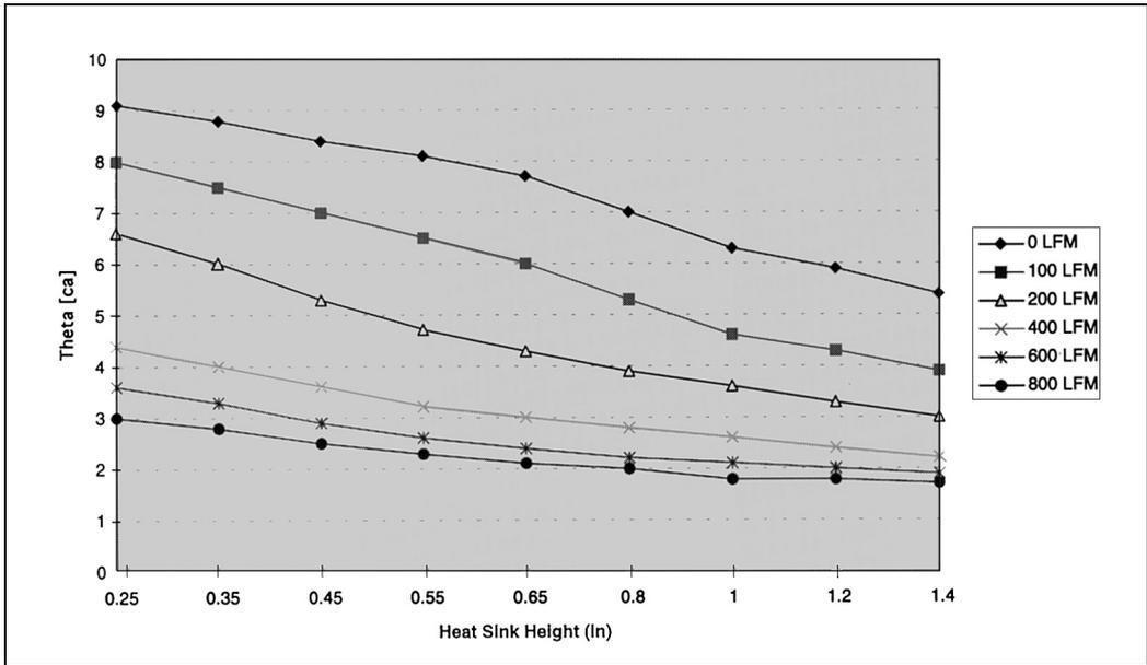
Figure 26-3. Thermal Resistance vs. Heatsink Height (Non-Spreader Package)
