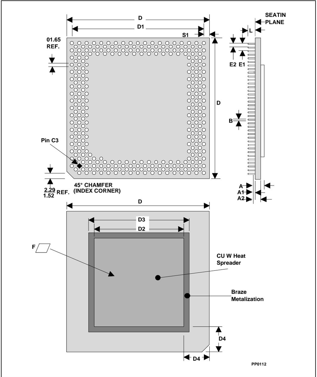
Figure 25-1. Package (with the heat spreader) Dimensions
