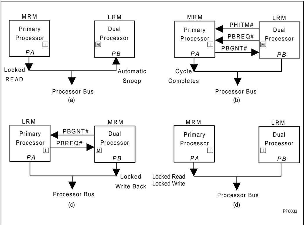
**Figure 20-6. DP Cache Consistency for Locked Accesses**
