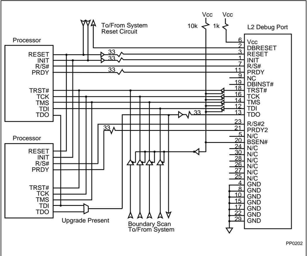
Figure 31-5. Dual CPUs — Boundary Scan Used
