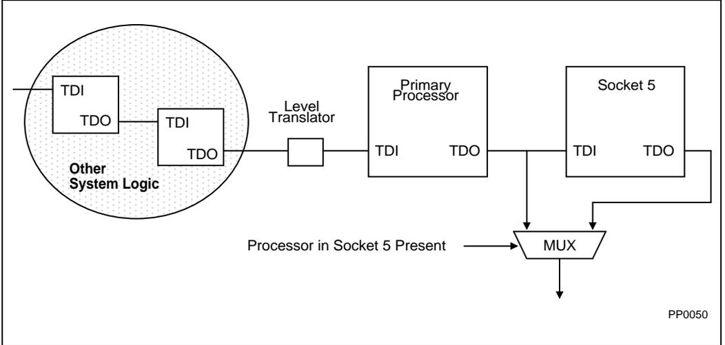
Figure 20-10. Dual Processor Boundary Scan Connections
