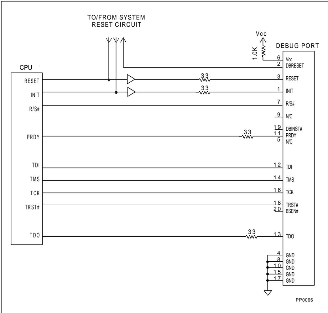
Figure 31-2. Single CPU — Boundary Scan Not Used
