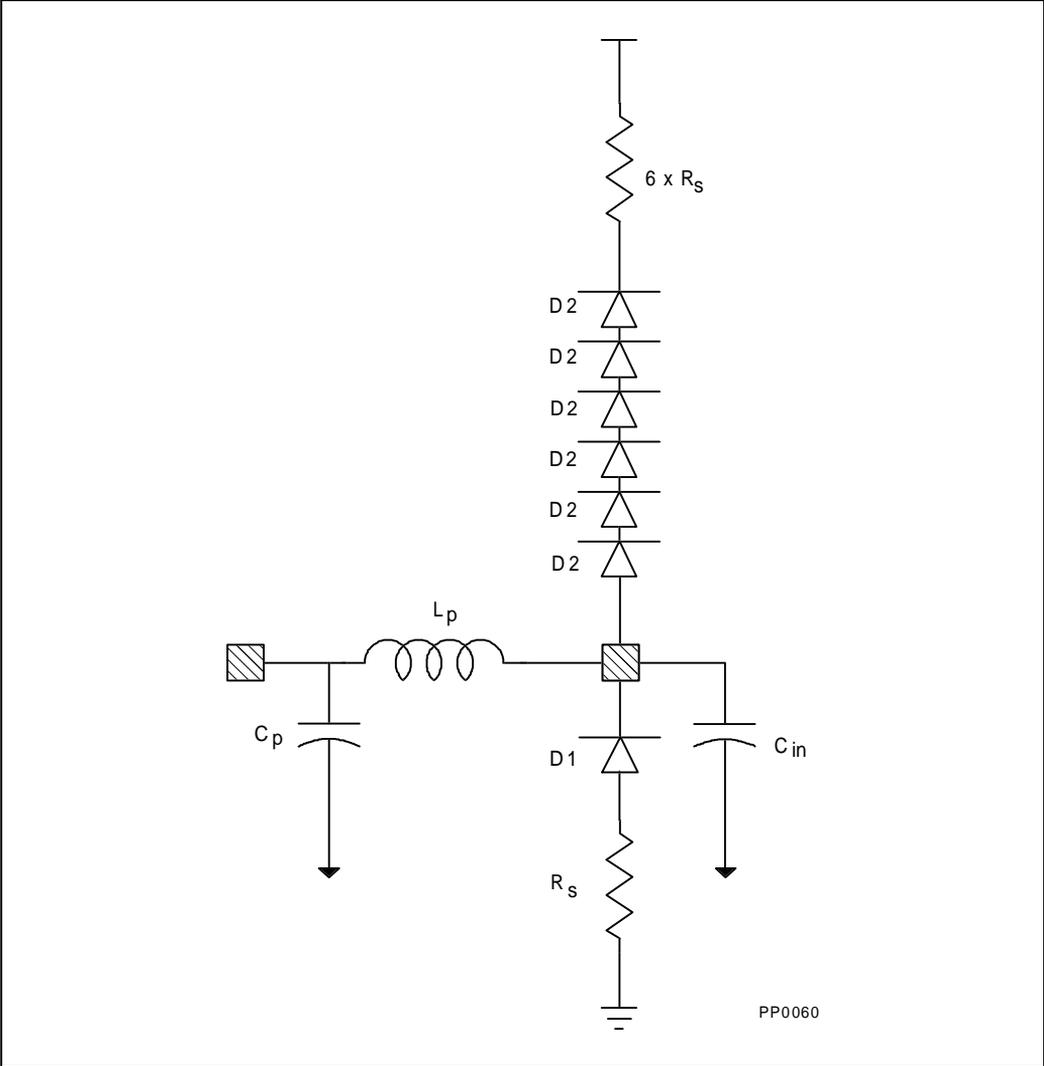
Figure 24-2. Input Buffer Model for Special Group
