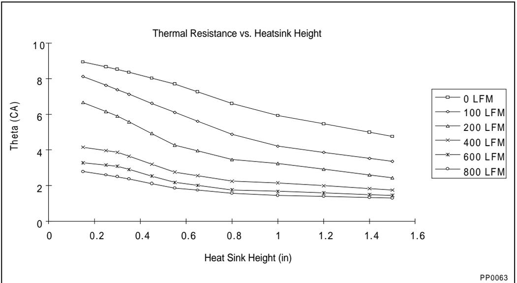
**Figure 26-2. Thermal Resistance vs. Heat Sink Height**
