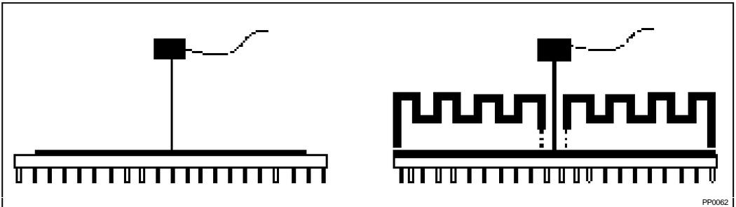
**Figure 26-1. Technique for Measuring  $T_C$ \***
