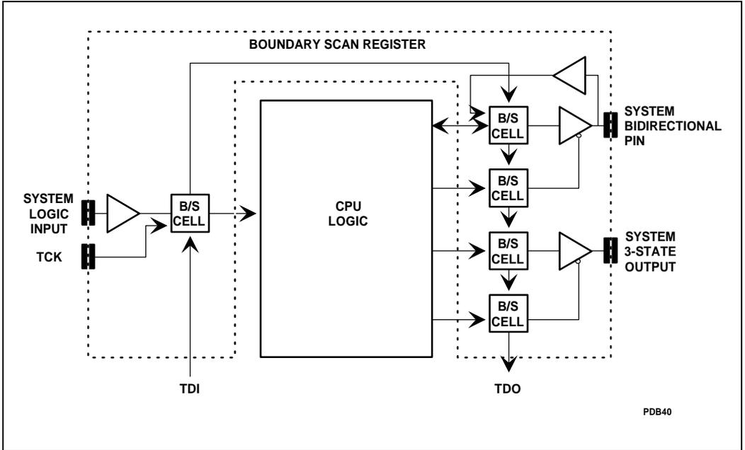
Figure 11-2. Boundary Scan Register
