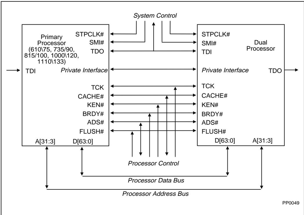
**Figure 20-9. Dual Processor Configuration**
