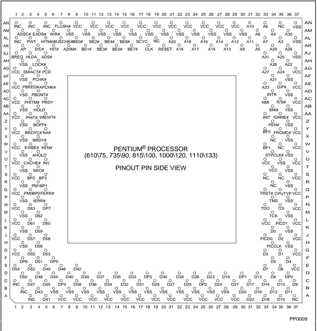
**Figure 17-2. Pentium® Processor (610\75, 735\90, 815\100, 1000\120, 1110\133) Pinout — Pin Side View**
