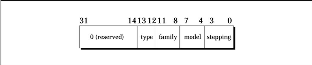
**Figure 20-1. EAX Bit Assignments for CPUID**
