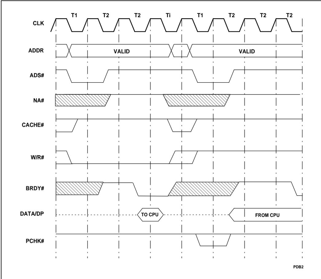
Figure 6-7. Non-Pipelined Read and Write with Wait States
