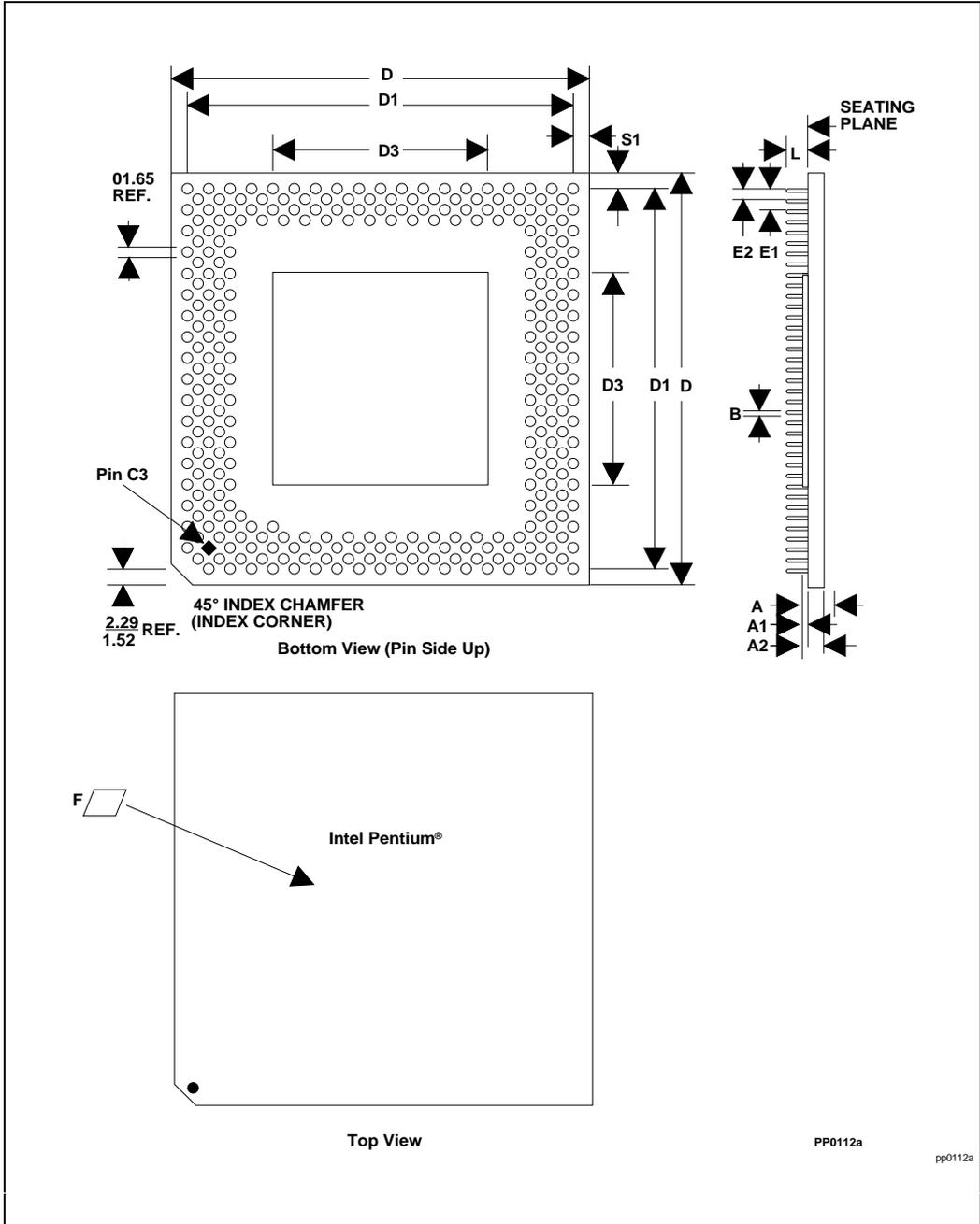
Figure 25-2. Package (without the heat spreader) Dimensions
