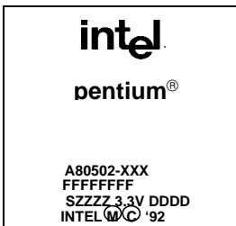
mcB1-Step Production SPGA Units:
