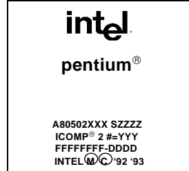
mA4-Step Engineering Sample SPGA Units:
