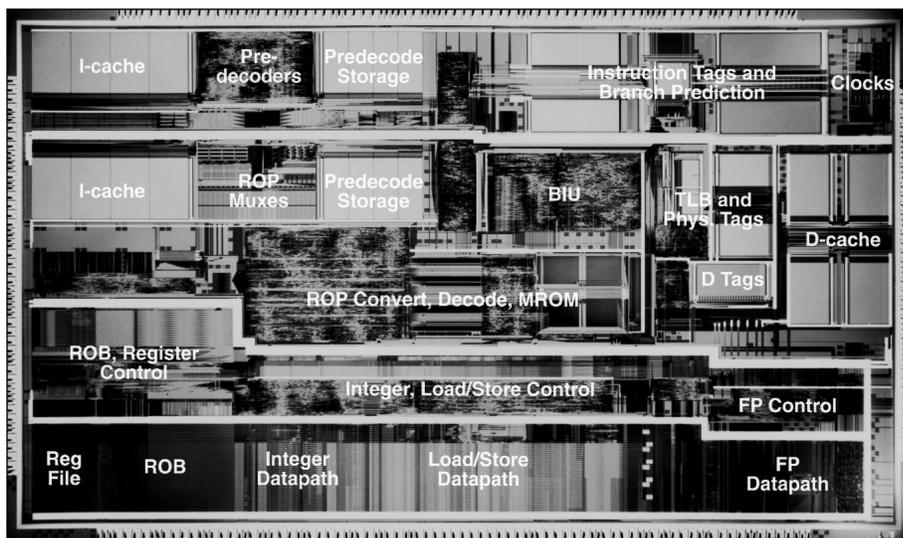
Figure 1. AMD's K5 incorporates 4.3 million transistors on a 251-mm<sup>2</sup> die using a 0.5-micron three-layer-metal CMOS process.
