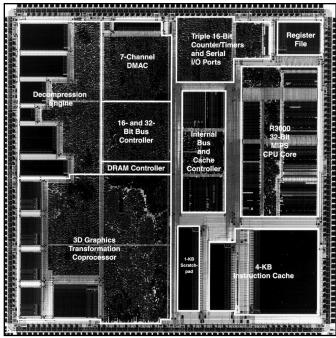
Figure 1. The custom CPU for the Sony PlayStation uses LSI's 0.5micron, three-metal-layer CMOS process and contains about one million transistors. LSI did not reveal the die size.
