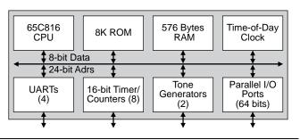
Figure 1. Western Design Center's 65C265 combines the 65C816 core with ROM, RAM, and I/O.
