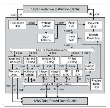
Figure 2. The Sparc64 CPU can issue up to four instructions per cycle, which are then executed by the decoupled function units.
