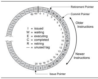
Figure 3. The Sparc64 uses 6-bit tags to ensure that instructions are retired in correct program order even when executed out of order.
