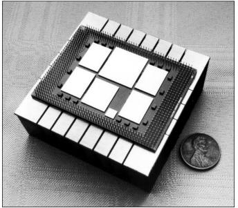
Figure 5. The Sparc64 module contains a large CPU chip and a smaller MMU chip surrounded by four identical cache chips and a tiny analog clock chip. The 565-pin ceramic PGA package measures  $6.1 \times 4.5$  cm, not including the large heat sink.
