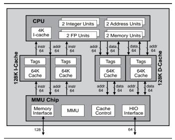
Figure 1. The Sparc64 processor consists of the CPU chip, the MMU (system-interface) chip, and four cache chips.
