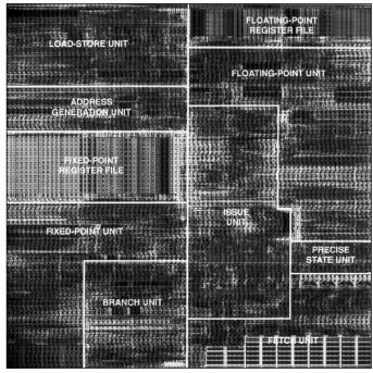
Figure 6. The Sparc64 CPU measures  $17.5 \times 16.9$  mm and consumes 2.7 million transistors in 0.4-micron four-layer-metal CMOS. There is no pad ring due to the flip-chip mounting process. The fetch unit includes a 4K instruction cache; the data cache is off chip.
