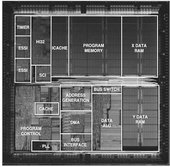
Figure 1. In Motorola's 0.5-micron three-layer-metal process, the 56301 measures about 7.6 mm on a side (58 mm<sup>2</sup>). The new 56300 core accounts for only a small portion of the total die area.
