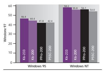
Figure 1. When tested in similar systems, AMD's 233-MHz K6 outscores a 200-MHz Pentium Pro and a 200-MHz Pentium/MMX on the Winstone 97 benchmark under both Windows 95 and Windows NT. See text for configurations. (Source: AMD)
