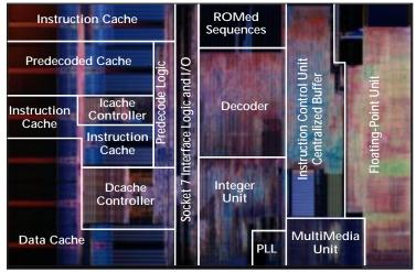
Figure 2. With 8.8 million transistors, the K6 measures  $15.7 \times 10.3$  mm when built in AMD's 0.3-micron five-layer-metal CS-34EX process.
