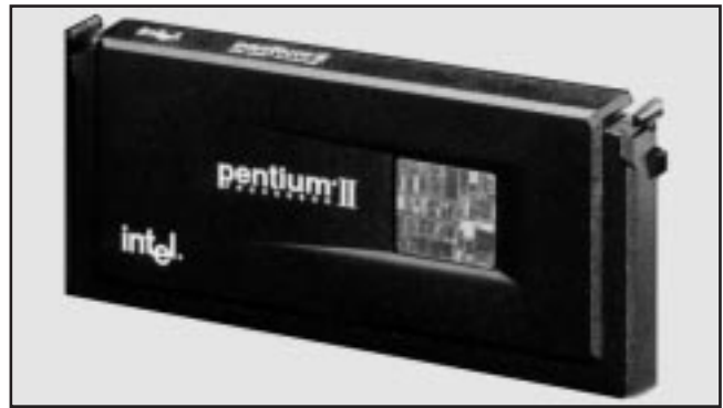
Figure 5. The PC board is enclosed in a plastic case measuring 5.73 x 2.47 x 0.66 inches. The case provides physical protection, EMI shielding, and a decorative hologram. In systems, a large heat sink will be mounted onto a metal plate on the rear (not shown).
