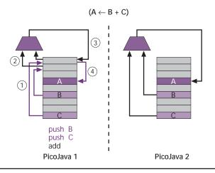
Figure 2. The PicoJava 2 core is more aggressive than the original PicoJava 1 in bypassing stack manipulation. The core's decode logic recognizes common stack operations and converts them to straightforward two-input ALU functions like a conventional CPU.
