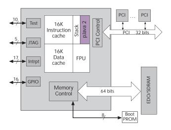
Figure 3. Sun's initial MicroJava 701 implementation will include a pair of 16K caches, a 64-bit memory controller, and a PCI bus.
