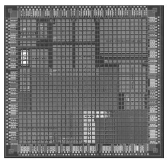
Figure 4. Die plot of proposed MicroJava 701 layout indicates the chip will measure about 50 mm<sup>2</sup> in a 0.25-micron CMOS process.
