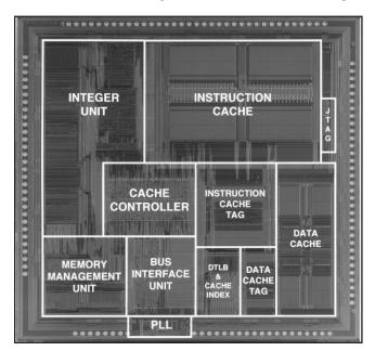
**Figure 1.** Die photo of the 29-mm<sup>2</sup> R32364 shows the large amount of area devoted to the 8K instruction cache and that the PLL encroaches on the pad ring.
