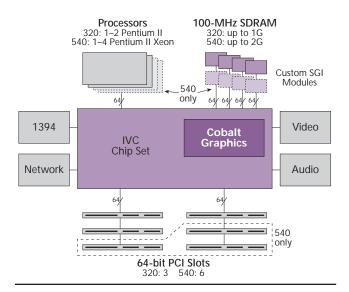
Figure 1. SGI's two new Windows NT workstations share the same architecture, which provides high bandwidth to main memory for all major subsystems.
