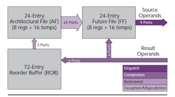
Figure 4. Athlon uses a future file to access source operands rather than the associative lookup used in classical reorder buffers.
