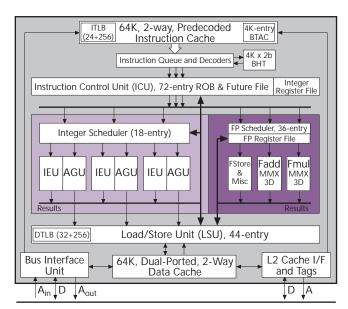
Figure 3. Athlon can decode up to three x86 instructions per cycle and issue up to nine ROPs per cycle out of order into its nine execution units. Up to 72 ROPs can be in flight at a time.
