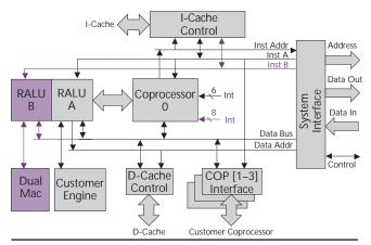
Figure 1. The LX5280 adds Radiax instructions and a new pipe to Lexra's earlier uniscalar LX4180.
