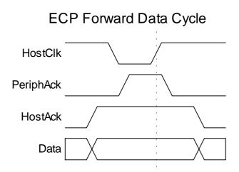
Figure 1. Enhanced Capabilities Port Forward Data Cycle.
