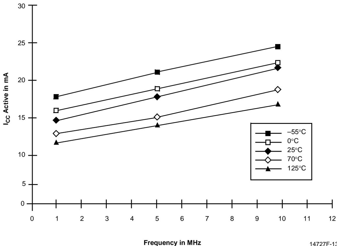
**Figure 5. Am28F020—Average I<sub>CC</sub> Active vs. Frequency**
