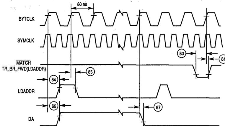
**Figure 13-12. CAM Interface Timing**
