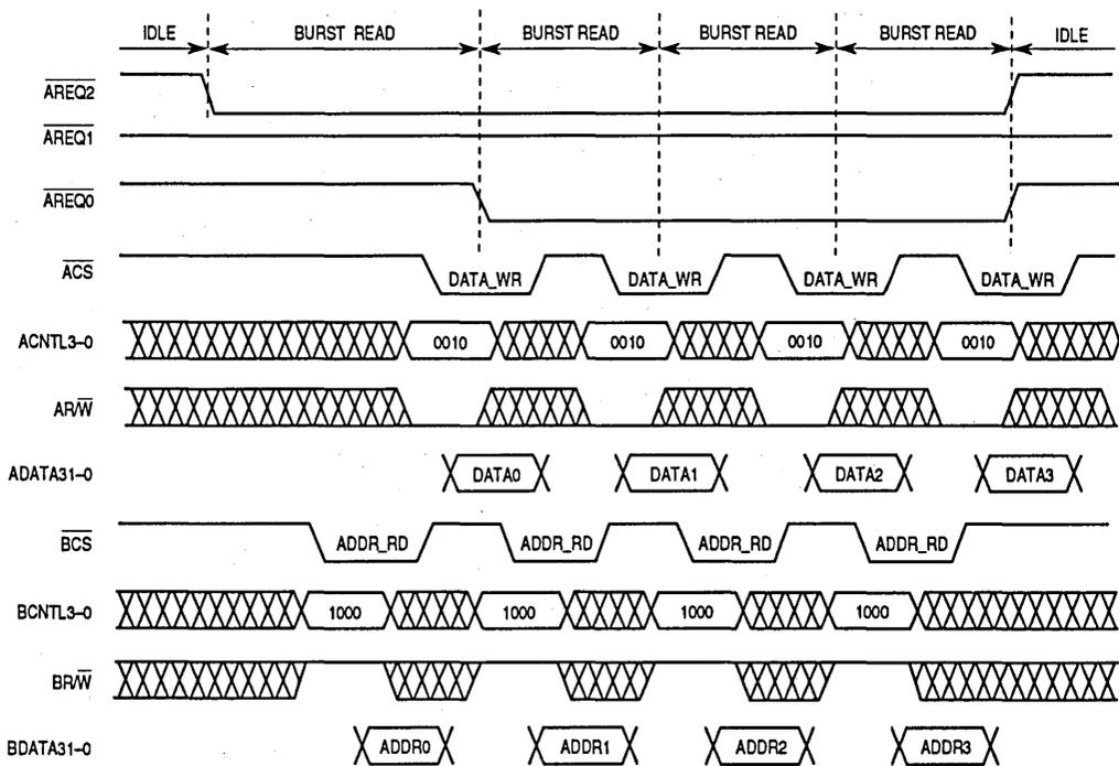
**Figure 6-4. Nonmultiplexed Address/Data Operation**
