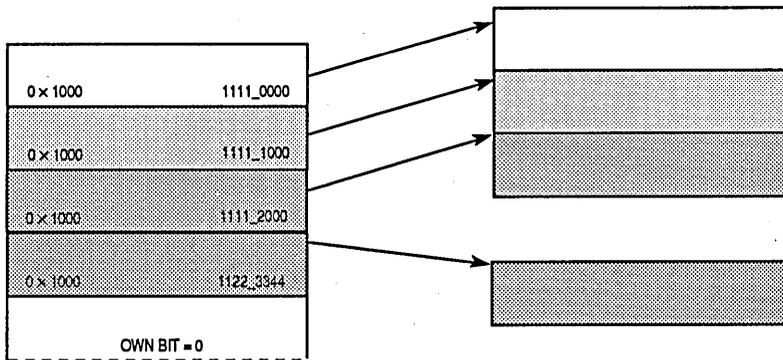
**Figure B-3. Descriptor Ring Pointer Structure**
