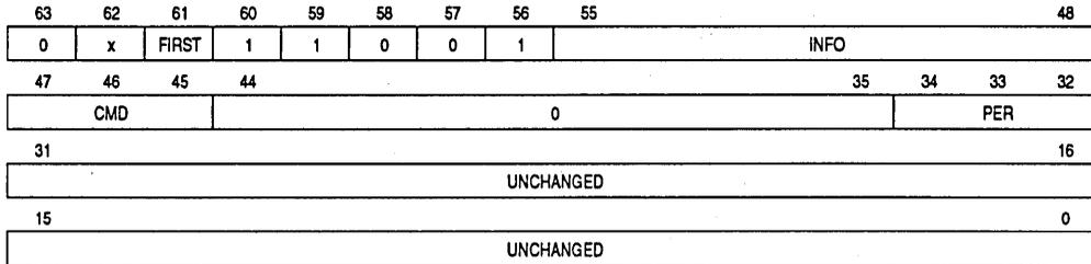
**Figure 9-15. DMA ERROR Indication (Destination Side)**
