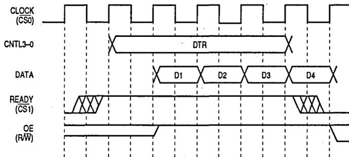
Figure 6-16. Pipeline Read without Wait State Timing
