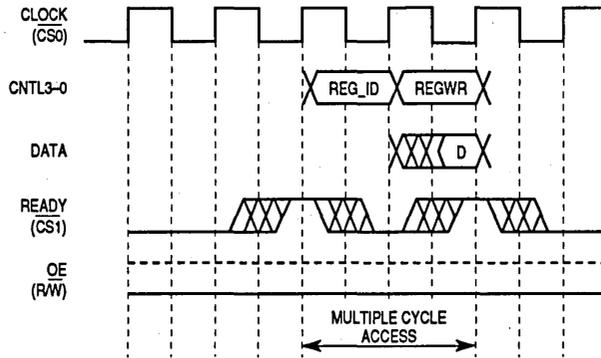
Figure 6-21. Register Write Timing
