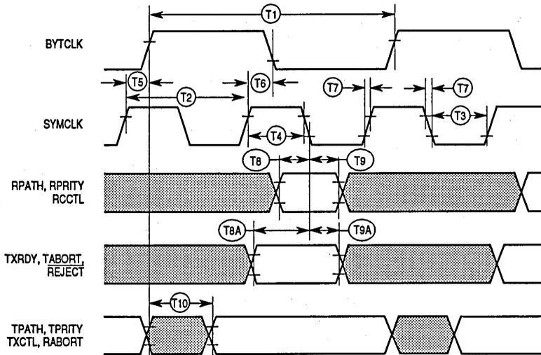
Figure 10-3. FSI Clocks and MAC Interface Timing
