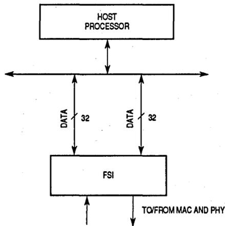
**Figure A-5. Slave Configuration with 64-Bit Data**
