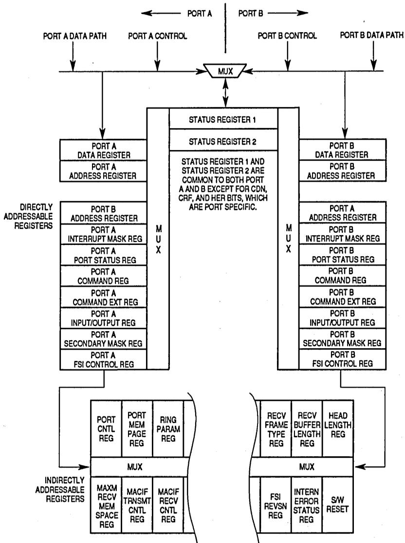
Figure 7-3. System Interface Block Internal and Common Registers
