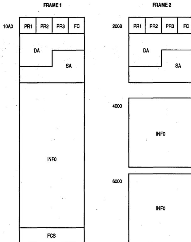
Figure 2-3. User Data Fields within System Memory
