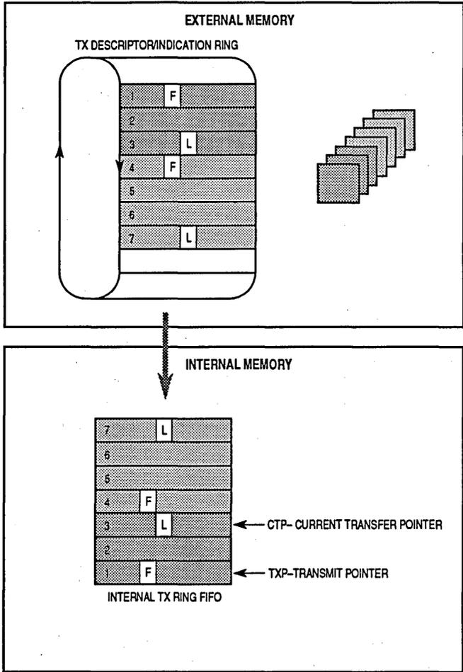
Figure 5-9. Internal Descriptor FIFO
