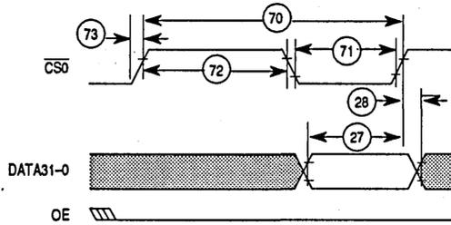
Figure 13-9. Pipeline Mode—FDDI Write
