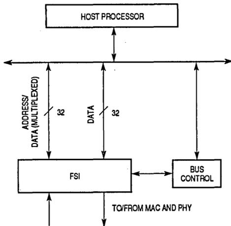
Figure A-6. 64-Bit Data with FSI DMA
