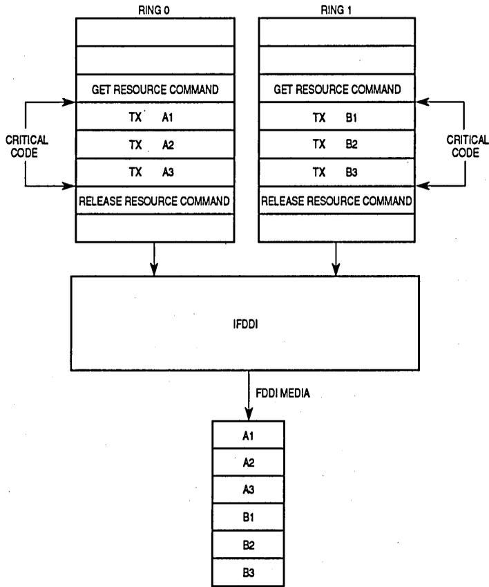
Figure 3-10. Example of Critical Code Protection
