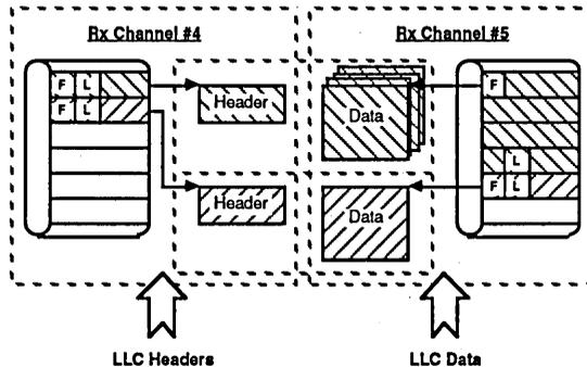
Figure 5-22. Header Splitting
