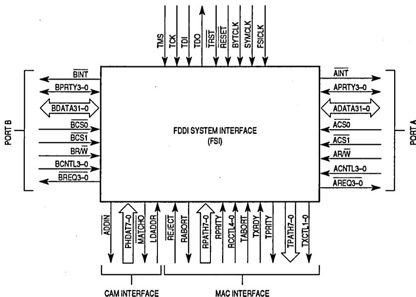
Figure 10-2. IFDDI Pinout in FSI Mode Only
