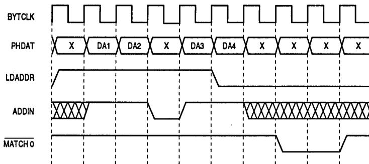
**Figure C-5. Four Bytes Comparison in Multiple Address Mode Using ADDIN**
