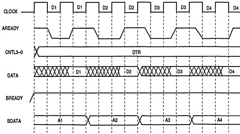
Figure 6-13. DMA Write to IFDDI - Read from DRAM (One Wait State)
