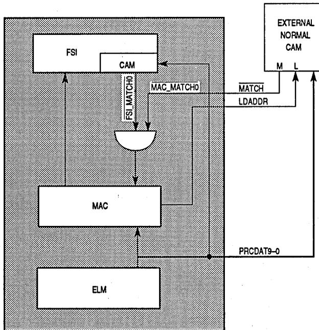
Figure 3-13. CAM Configuration in Normal Match Mode
