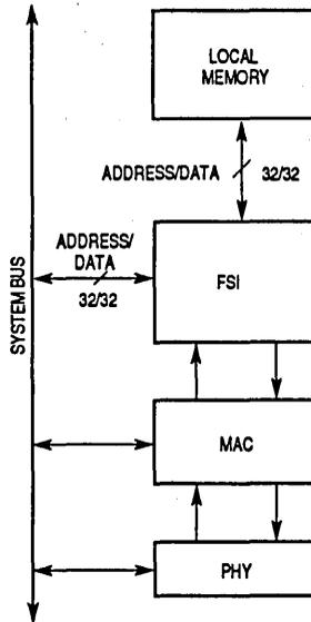
**Figure A-3. Basic Configuration with Local Memory**
