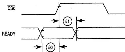
**Figure 13-11. Pipeline Mode—READY Input**
