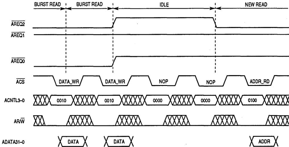
Figure 6-5. Synchronous Operation
