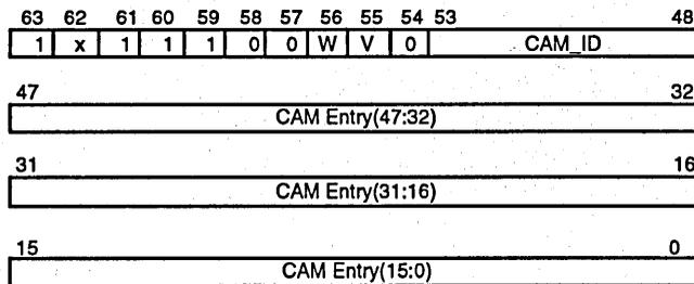
Figure C-6. Set Up CAM Command
