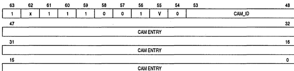
Figure 9-25. SET UP CAM Command
