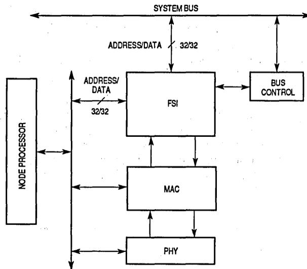
**Figure A-2. Basic Configuration with Separate Node Processor**
