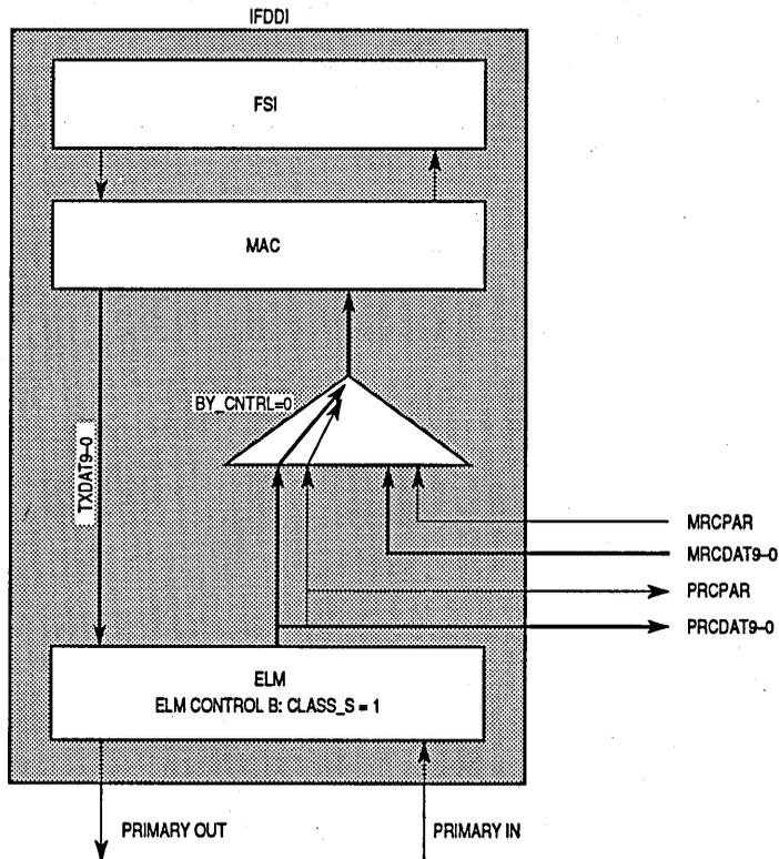
Figure 3-11. Single Attach Station
