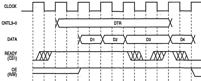
**Figure 6-17. Pipeline Read with Wait State Timing**
