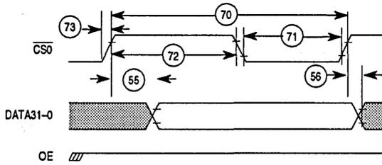
Figure 13-8. Pipeline Mode—FDDI Read
