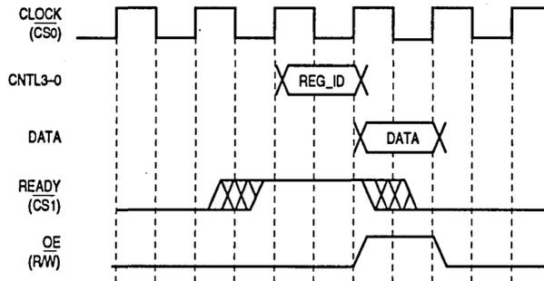
**Figure 6-20. Register Read Timing**
