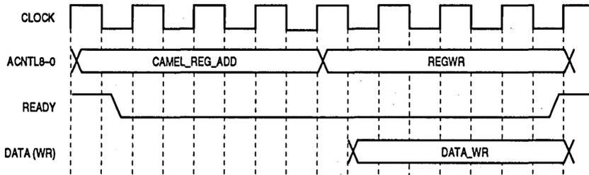
**Figure 6-23. Write CAMEL Internal Register In Pipeline Mode**
