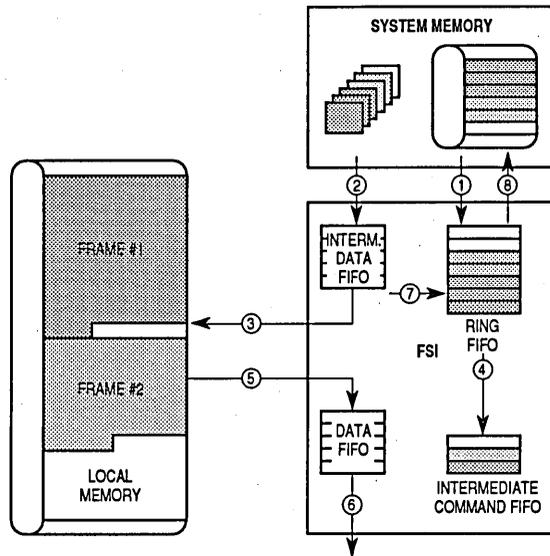
**Figure 5-17. Transmit Process**
