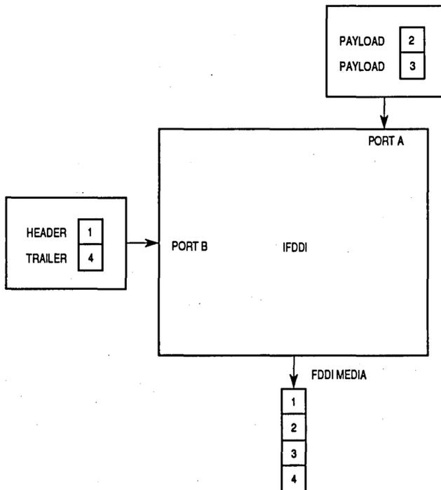
Figure 3-9. Continuous Frame from Fragmented Buffers
