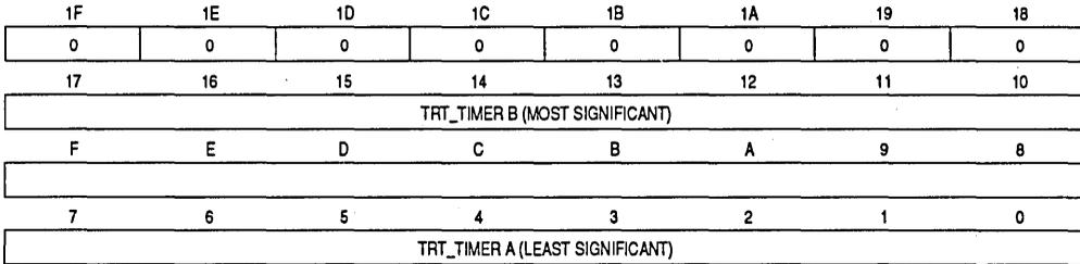
**7.3.12.3 THT TIMER AND SENT COUNT REGISTER (THT\_TIMER\_A, THT\_TIMER\_B, & SENT\_COUNT) ACNTL = 1 0110 1110; ACNTL = 1 0110 1111.** Since the THT timer is 24 bits, it may need to be read in two consecutive reads (only when  $T\_Opr$  is  $\geq 5.242880$  ms). Because this register can (and usually will) change between the two read operations, care must be taken to get a consistent value.
