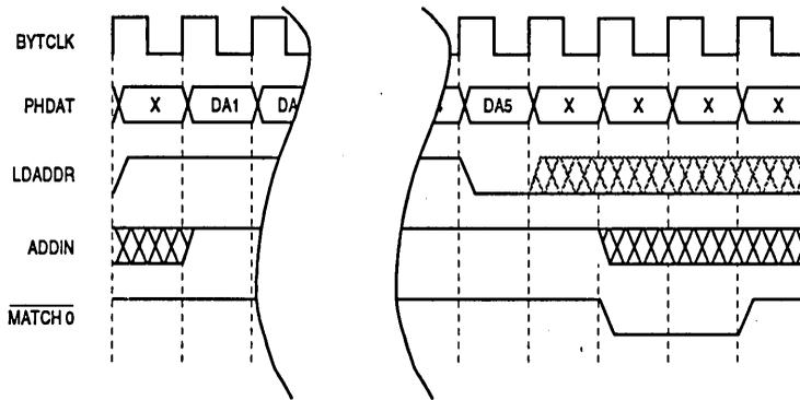
**Figure C-3. CAM Operation in Multiple Address Mode**
