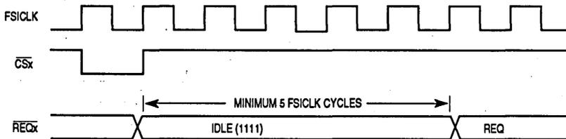
**Figure 6-8. Request Negation to Request Assertion in Asynchronous Mode**
