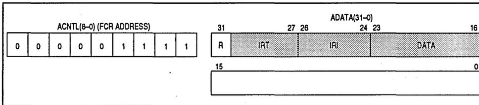
NOTE: IN FCR READ OPERATIONS, THE DATA TO BE READ IS VALID ON ADATA(23-16) WHEN THE CONTROL REGISTER FREE BIT IN STATUS REGISTER 1 IS SET TO ONE AFTER A READ OPERATION IS REQUESTED. BIT 31 SHOULD BE EQUAL TO ONE WHEN REQUESTING A READ FROM THE FCR AND SHOULD BE ZERO WHEN PERFORMING A WRITE OPERATION.
