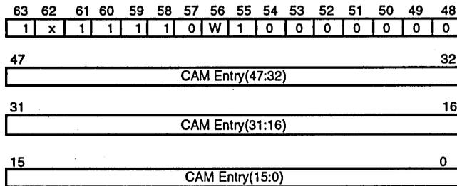
Figure C-8. Compare CAM Entry Command
