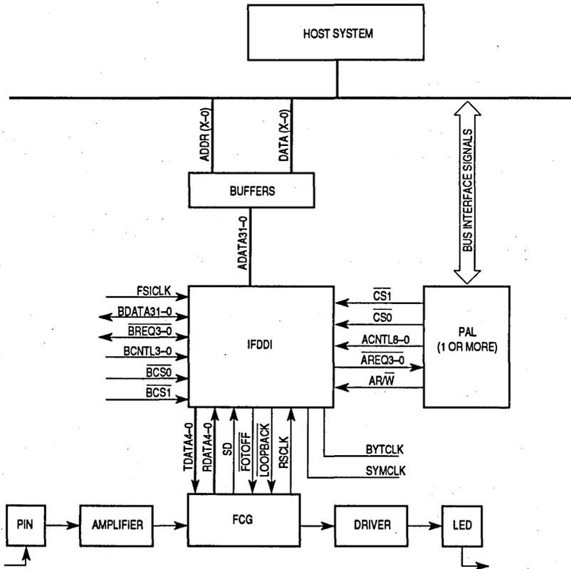
Figure 2-1. Basic System Configuration
