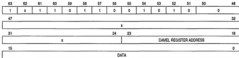
Figure 9-32. 16-BIT CONTROL REGISTER WRITE Command
