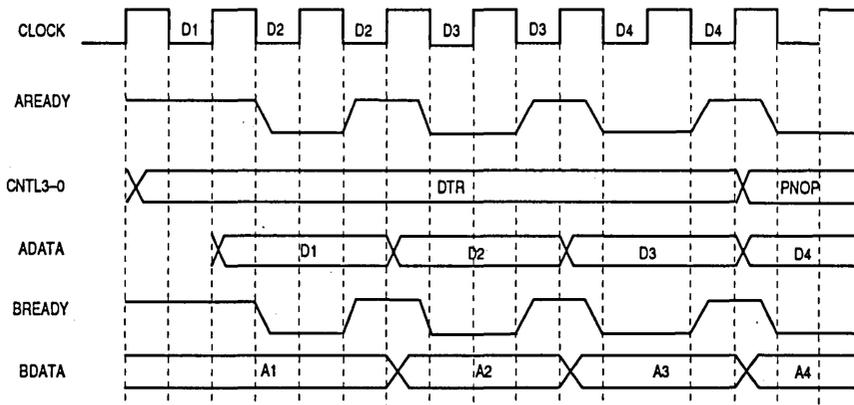
Figure 6-15. DMA Read from IFDDI - Write to DRAM (One Wait State)
