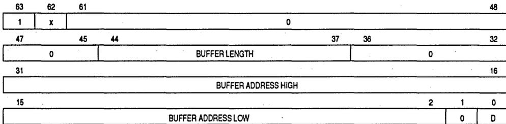
**Figure 9-18. Receive Buffer Descriptor**
