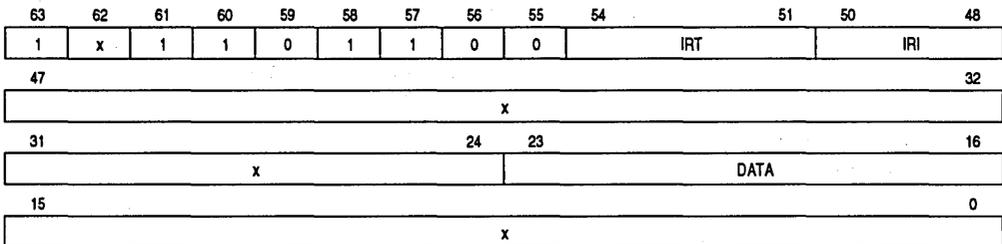
Figure 9-31. CONTROL REGISTER WRITE Command
