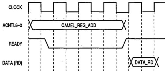
Figure 6-22. Read CAMEL Internal Register in Pipeline Mode
