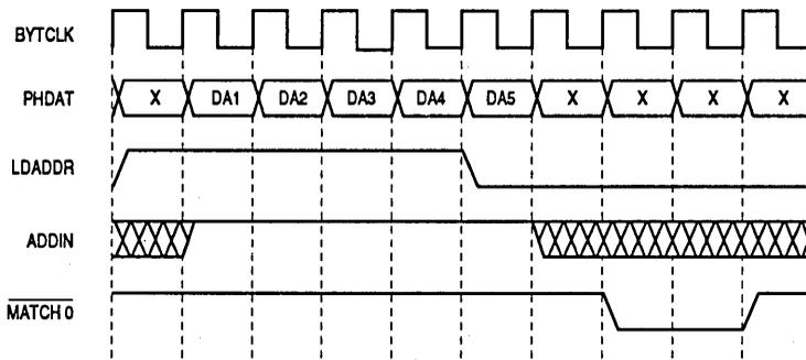
**Figure C-4. Five Bytes Comparison in Multiple Address Mode Without Using ADDIN**
