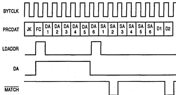
Figure 5-24. CAM Interface Signals (EXT\_DA\_MATCH = 0)
