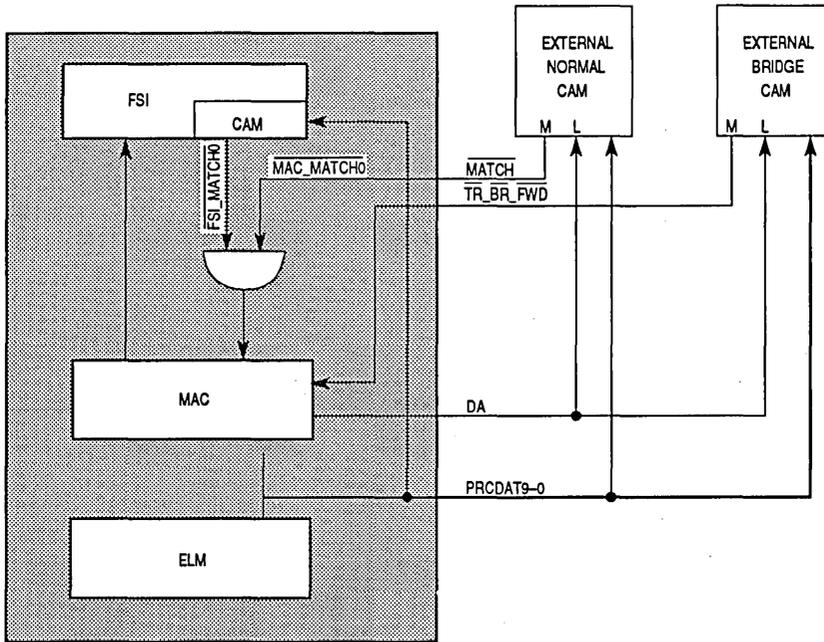
Figure 3-14. CAM Configuration in Extended Match Mode
