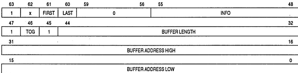
**Figure 9-11. DMA BUFFER DESCRIPTOR Command**
