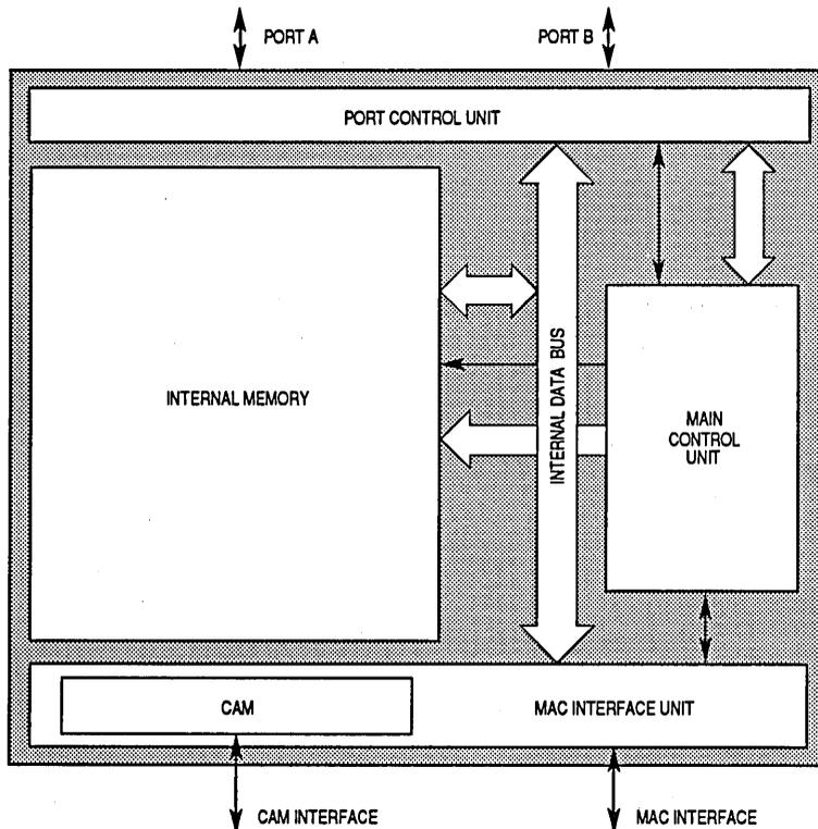
**Figure 4-2. FSI Internal Architecture**
