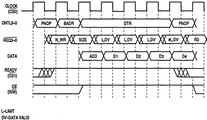
**Figure 6-24. Burst Read Cycle Timing**
