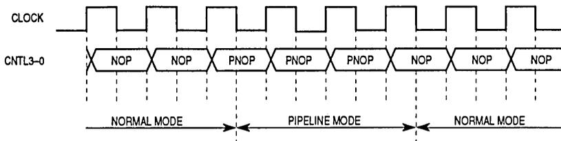
**Figure 6-10. Pipeline Mode Selection**
