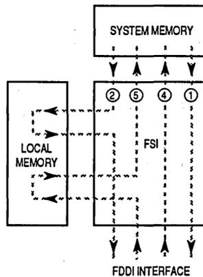
**Figure 5-3. Direct and Expanded Local Memory Options**
