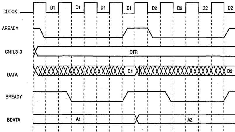
Figure 6-12. DMA Write to IFDDI - Read from DRAM (Multiple Wait States)
