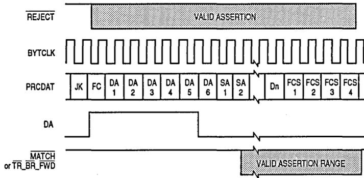
Figure 5-25. CAM Interface Signals (EXT\_DA\_MATCH = 1)
