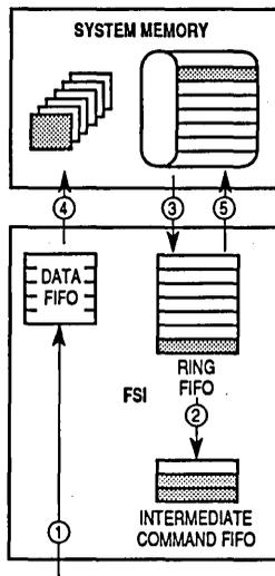
**Figure 5-14. Normal Reception by Ring Operation**
