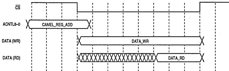
Figure 6-2. Read and Write CAMEL Internal Register Timing
