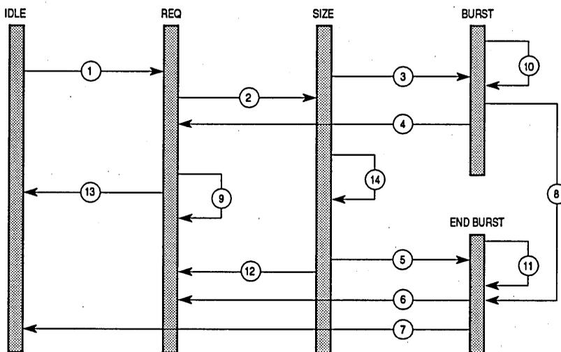
**Figure 6-11. IFDDI States During Burst Cycle**
