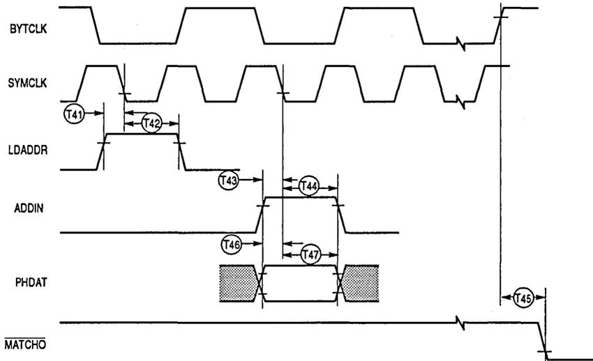
Figure 10-4. FSI-CAM Interface Timing
