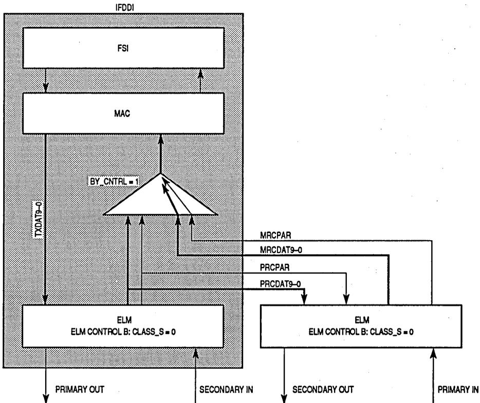
Figure 3-12. Dual Attach Station
