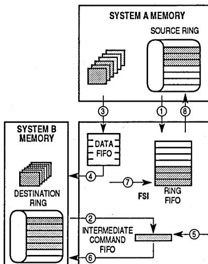
**Figure 5-20. DMA Operation for a Transmit Channel**
