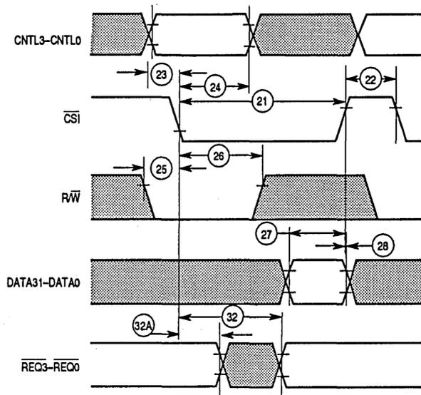
Figure 13-3. FSI Write Timing
