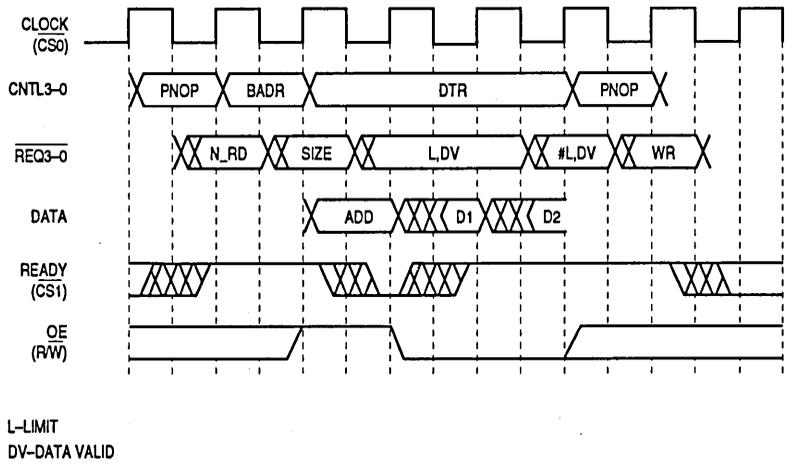
**Figure 6-25. Burst Write Cycle Timing**
