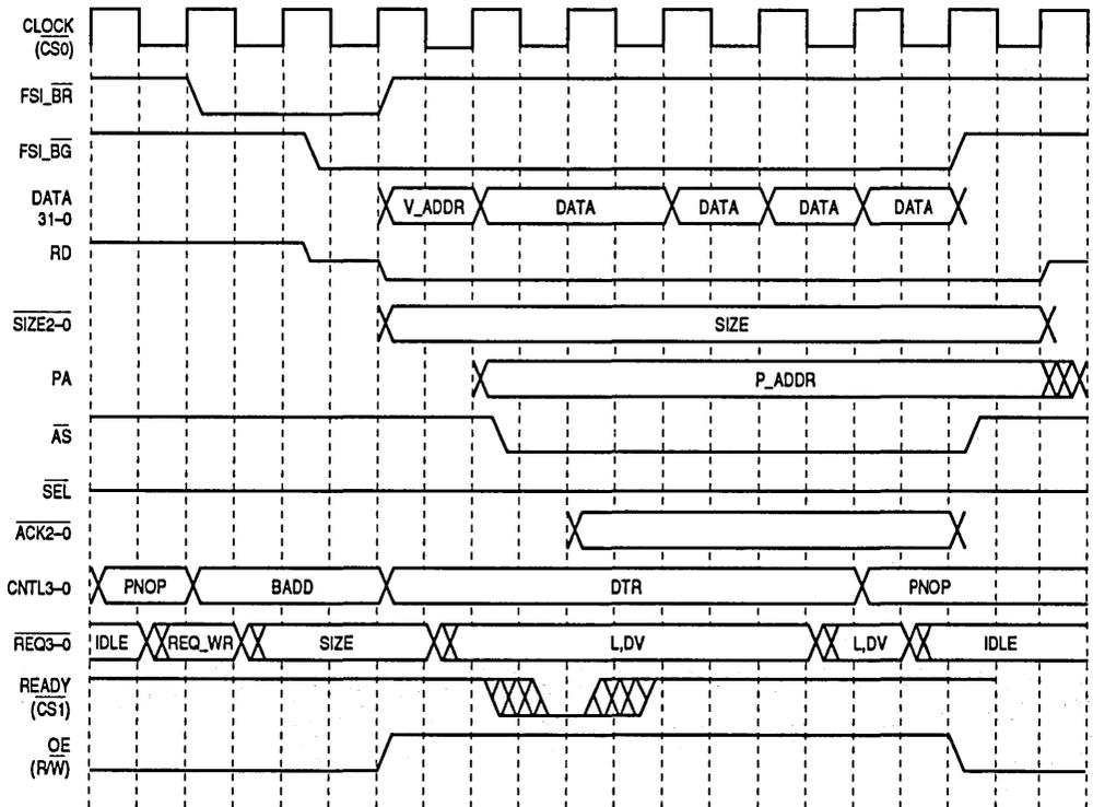
Figure 6-27. S-Bus Write Cycle (FSI Read Cycle)
