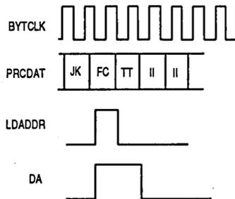
Figure 5-26. CAM Interface Timing (Receiving Token Frame for Normal and Extended Match Mode)
