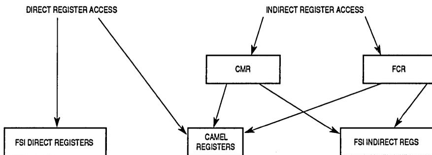
Figure 7-1. Register Access Methods
