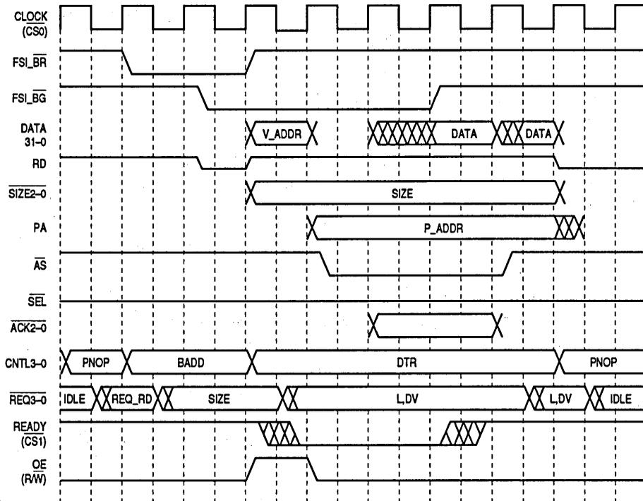
Figure 6-26. S-Bus Read Cycle (FSI Write Cycle)
