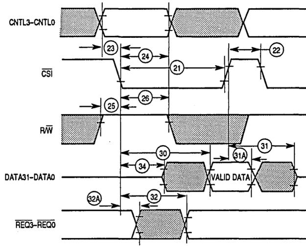
Figure 13-2. FSI Read Timing
