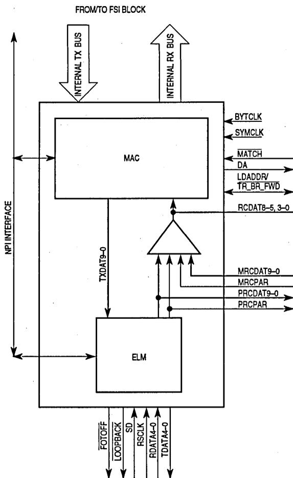
Figure 4-3. CAMEL Block Diagram
