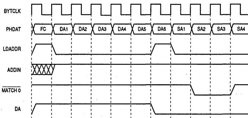
Figure C-2. CAM Operation in 48-bit Address Mode
