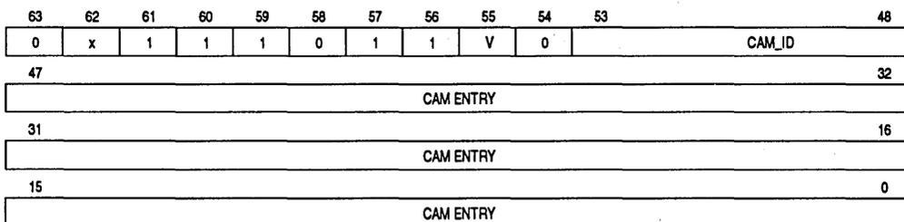
Figure 9-27. READ CAM ENTRY Indication
