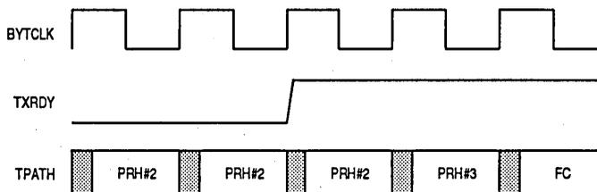
**Figure 10-1 TXRDY and Packet Request Header Timing**
