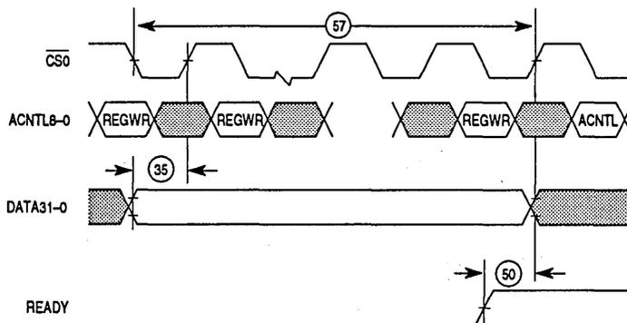
**Figure 13-6. CAMEL Direct Access Write Cycle (Pipeline Mode)**
