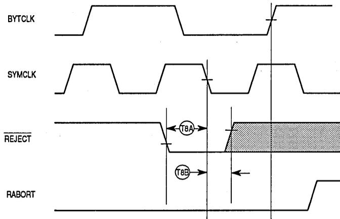
Figure 10-5. FSI  $\overline{\text{REJECT}}$ /RABORT Timing
