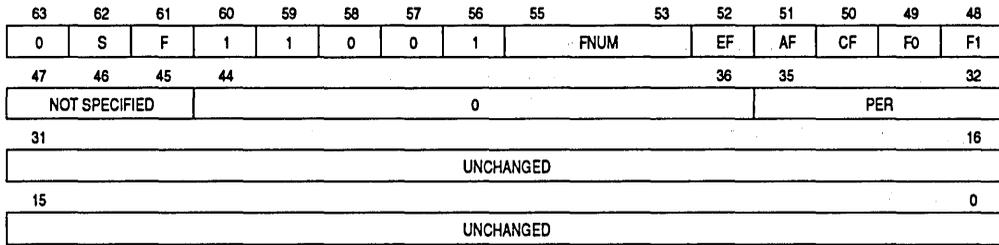
**Figure 9-21. RECEIVE PORT ERROR Indication**
