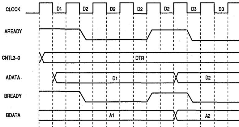
Figure 6-14. DMA Read from IFDDI - Write to DRAM (Multiple Wait States)
