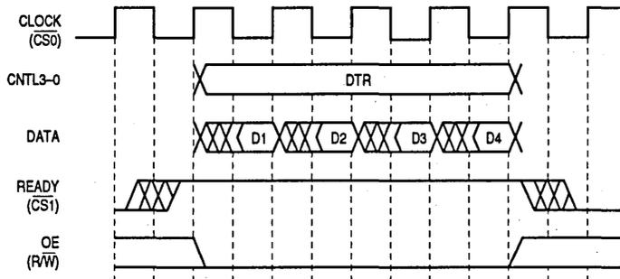
**Figure 6-18. Pipeline Write without Wait State Timing**
