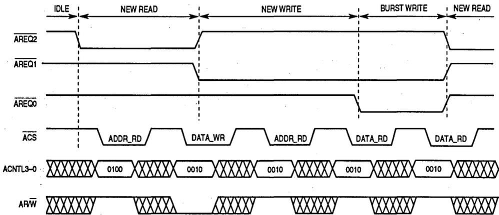
**Figure 6-7. Data Read Followed by a Data Write in the Same Bus Tenure**
