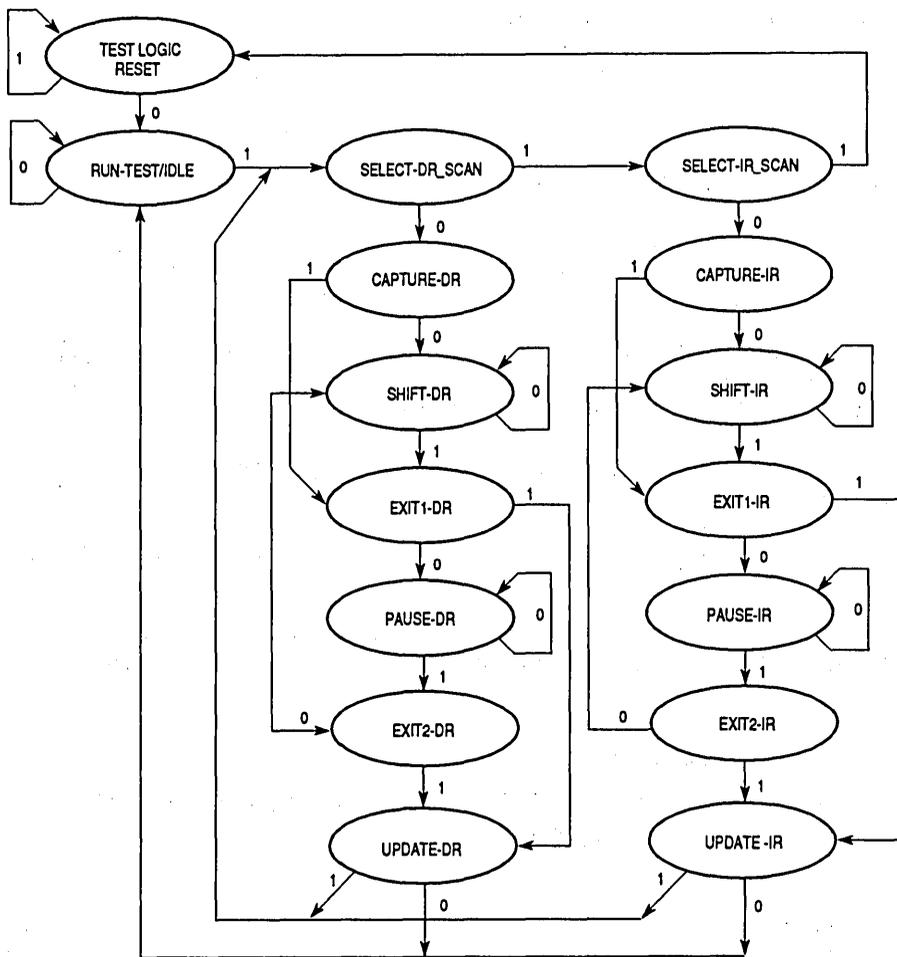
**Figure 12-2. TAP Controller State Machine**
