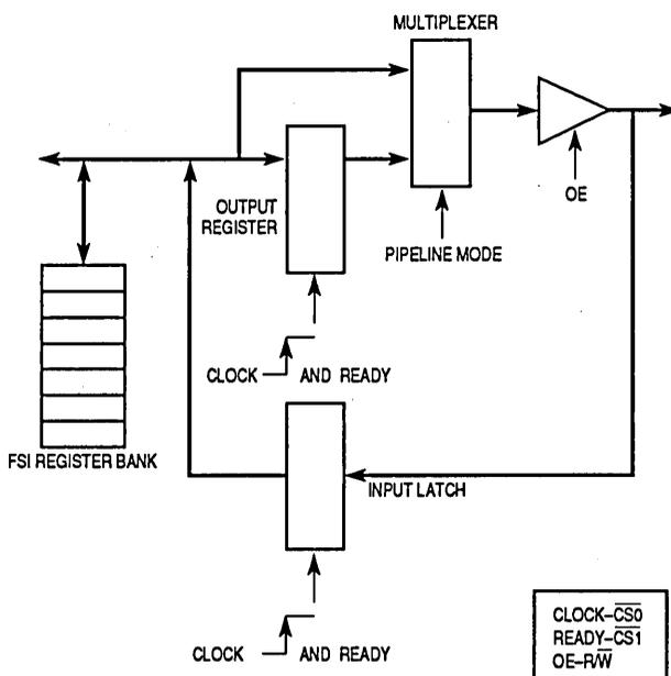
Figure 6-9. IFDDI I/O Basic Structure
