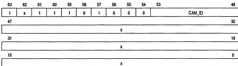
Figure 9-26. READ CAM ENTRY Command
