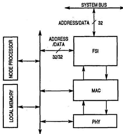
**Figure A-4. Local Memory with Separate Node Processor**
