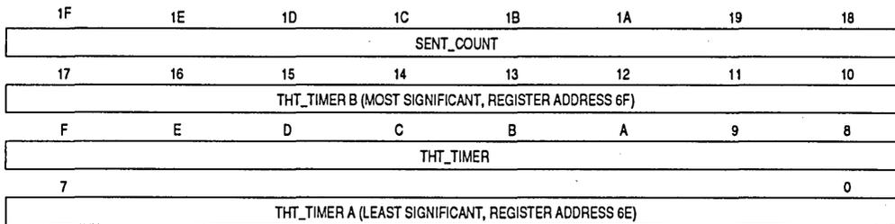
**7.3.12.4 NEGOTIATED TTRT REGISTER (T\_NEG\_A, T\_NEG\_B) ACNTL = 1 0110 0110; ACNTL = 1 0110 0111.** T\_NEG is a 24-bit read-only register that the node processor may need to read in two consecutive reads. Because this register can (but usually will not) change between the two read operations, care must be taken to get a consistent value.
