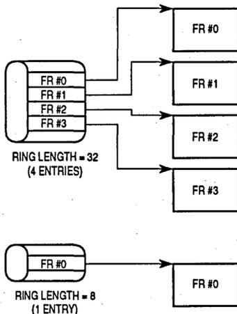
Figure 5-13. Endless Repeat of Data Frame Transmission
