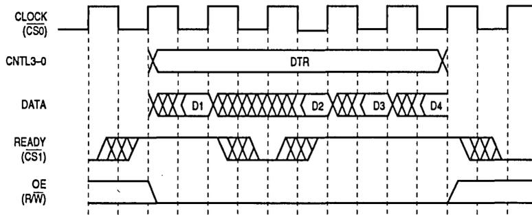
**Figure 6-19. Pipeline Write with Wait State Timing**
