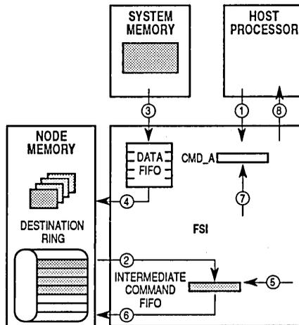
Figure 5-21. DMA Transfers Using Command Register
