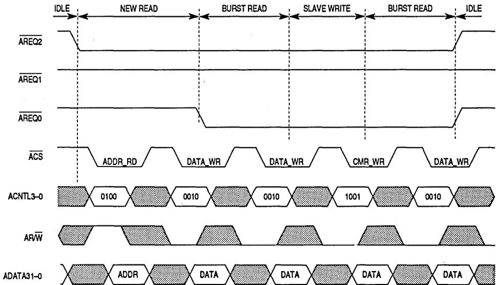
Figure 2-5. Basic Bus Cycle Example
