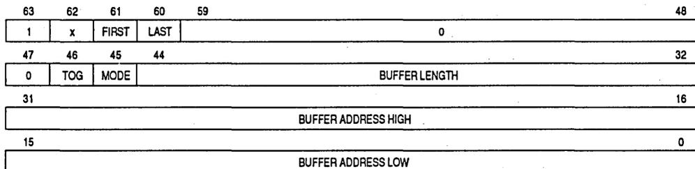
**Figure 9-9. TRANSMIT BUFFER DESCRIPTOR Command**
