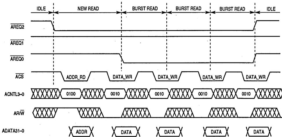
**Figure 6-3. Address/Data Multiplexed Operation**
