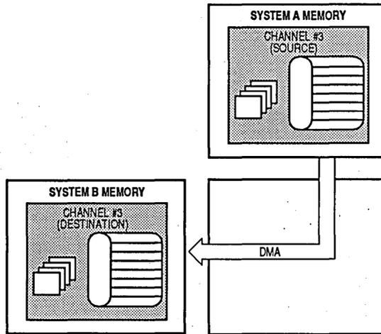
**Figure 5-19. Port to Port DMA**
