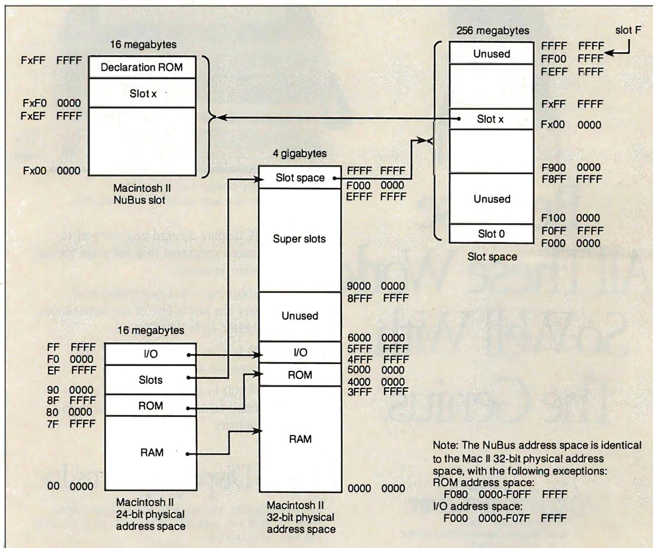
Figure 2: The Macintosh II memory map. The memory in the superslot space and 15 megabytes of the slot space are not available to the Macintosh II, but NuBus cards can access these regions.
