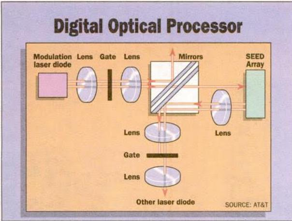
Each array contains two modulated laser diodes divided into separate beams that provide communications between arrays.
