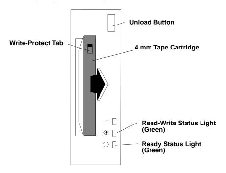
The time required for a tape to rewind and unload is between 10 seconds and 1.5 minutes, depending on the position of the tape when the unload button is pushed.
