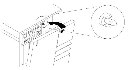
4. On the rear of the unit, turn the locking handle counterclockwise 90 degrees to lock the front cover.
