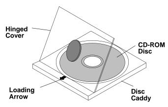
With the loading arrow toward the drive and the printed side of the disc up, insert the caddy in the disc caddy opening. Push gently on the caddy. The drive automatically pulls the caddy into the drive and prepares the disc for reading.
