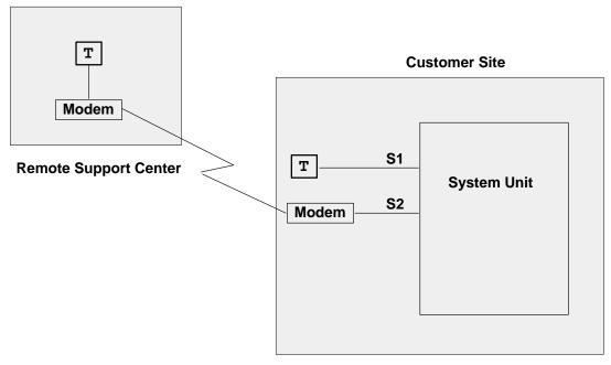
When mirroring is active, the customer on the BUMP Console and the support personnel on the Service Console both see the same output on their screens, and either one may enter characters. One person can even start typing and the other finish it. For example, the support personnel may log in as root on the Service Console, and the customer may enter the root password on the BUMP Console. Therefore, the remote support personnel do not need to know the root password.
