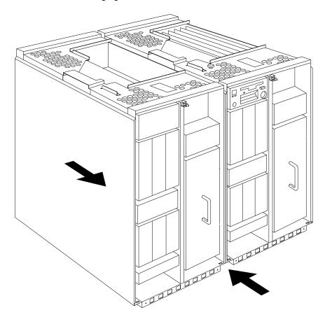
1. Start the screw through the hole in the locking bar and into the hole located in the lower right corner of the left unit, as illustrated in the figure. Push the locking bar against the units.
