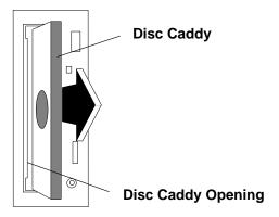
If the disc caddy cannot unload and has to be removed manually from the drive, contact your service representative.
