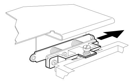
7. Secure the mechanics of the FXE cable to the base unit back plane mechanical support tightening clockwise the screw illustrated in the figure.
