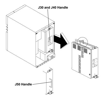
2. Remove the metal bridge from the base unit,in the area circled in step 4.
