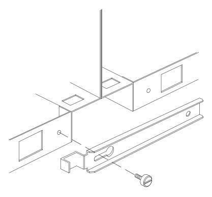
2. Slide the locking bar to the right and start the screw through the hole of the locking bar and into the unit on the left, as shown.
