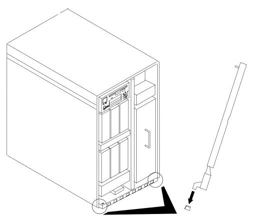
3. When the pins are in place push the cover closed until the retaining clip catches the locking pin. The locking pin must be in the position shown in the figure.
