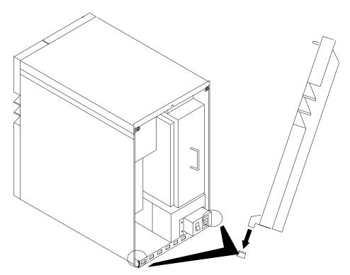
3. When the pins are in place, close and lock the rear cover.
