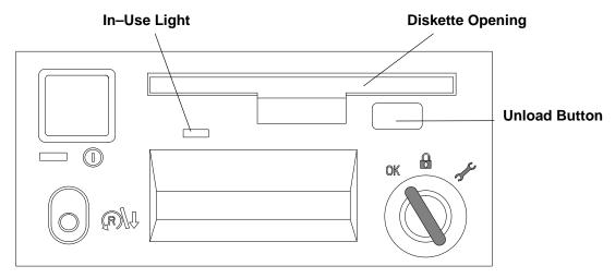
**Unload Button** Used to unload the diskette from the drive
