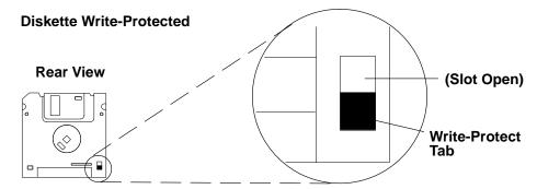
To enable writing onto a diskette, slide the write-protect tab to cover the protect slot.
