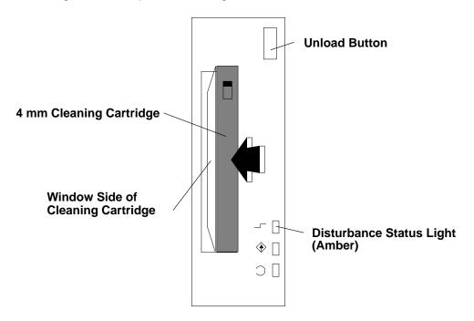
After the 4 mm cleaning cartridge has been fully inserted into the 4 mm tape drive, the following cleaning operations are performed automatically:
