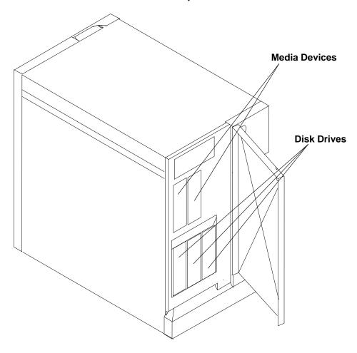
Nine slots for 3.5-inch disk drives are located in the rear of the expansion unit.
