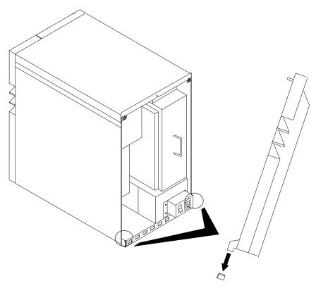
2. When the pins are in place, close and lock the rear cover.
