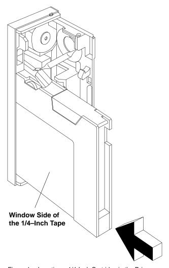
Figure 1. Inserting a 1/4-Inch Cartridge in the Drive
