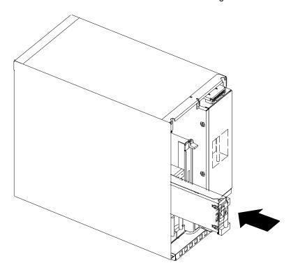
2. Insert the two positioning pins located on the lower edge of the rear cover into the corresponding holes of the unit.
