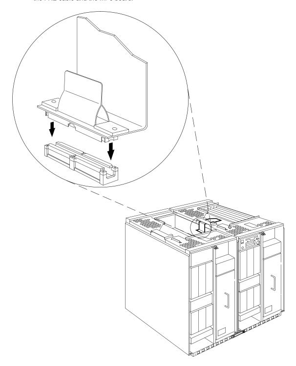
9. Replace the metal bridge as shown here. Use the new bridge that is shipped with the expansion unit (the side piece is shorter, to allow the FXE cable to fit under it). Be sure to attach the ground cable from the expansion unit to the base unit.
