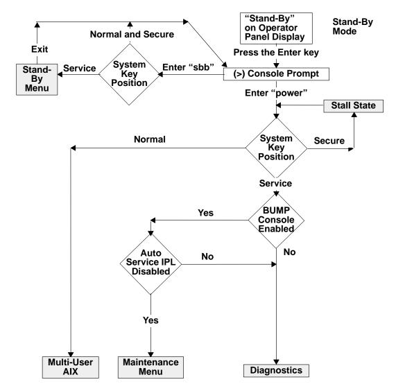
When the system is in Stand-By mode and the System Key (Physical or Electronic Key) is in Service mode, the STAND-BY MENU can be accessed and SystemGuard executed.
