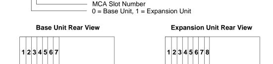
For example; 00–14–00–30 is the adapter in MCA slot 4 of the expansion unit.
