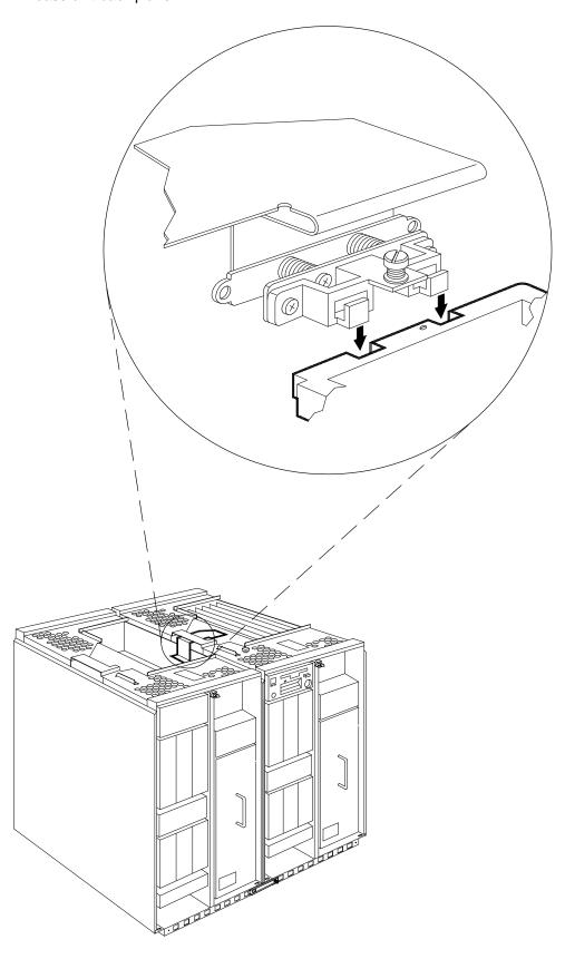
6. Slide the mechanics of the FXE cable following the direction shown in the figure.
