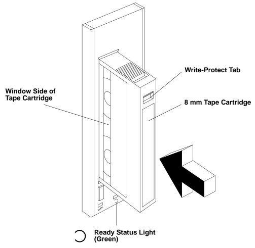
The tape takes about 25 seconds to load. When the green light comes on, the drive is ready for data operations.
