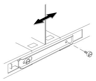
4. Using a screwdriver, tighten the screws clockwise as shown in the figure, to secure the locking bar.
