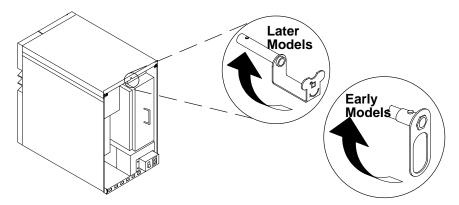
4. Tilt the front cover towards you and pull the cover up to remove it from the unit as shown in the figure.
