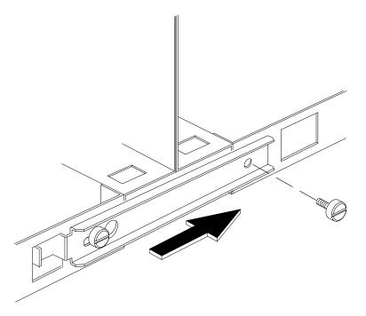
3. Pull the units apart, until locking bars stop you. This allows the doors to open and close smoothly.
