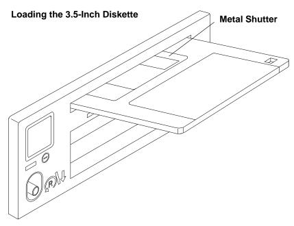
Push the diskette into the drive until you hear a click. The click indicates that the diskette is securely positioned in the drive.
