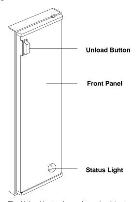
The Unload button is used to unload the tape from the drive.
