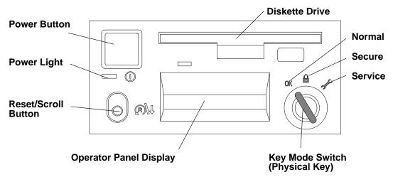
In the 7013 J Series the I/O card contains the NVRAM while the NVRAM battery and the TOD (Time-Of-Day) are located in the Operator Panel. You can drain NVRAM in the following ways:
