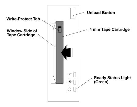
The 4 mm tape drive is ready for data operations when the tape cartridge is inserted. After the cartridge is inserted into the tape drive, the tape takes about 15 seconds to load.
