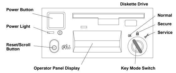
**Power Button** Used to switch the power to the system on or off
