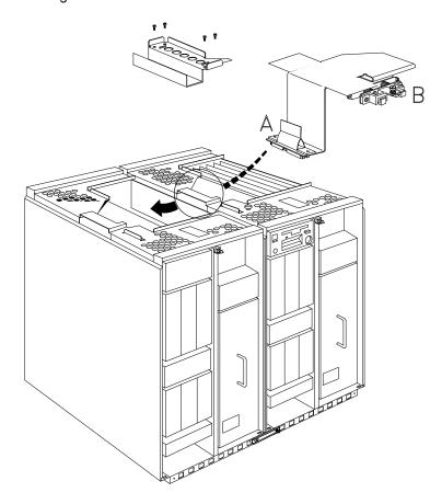
5. Insert the mechanics of the FXE cable into the mechanical support located in the rear of the base unit back plane.
