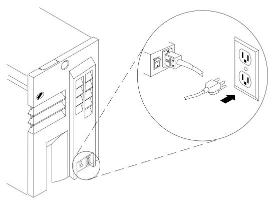
4. Perform this step first on the expansion unit if there is one attached. Press the switch located on the Main Power Switch Module to on, switching it to the "I" position.
