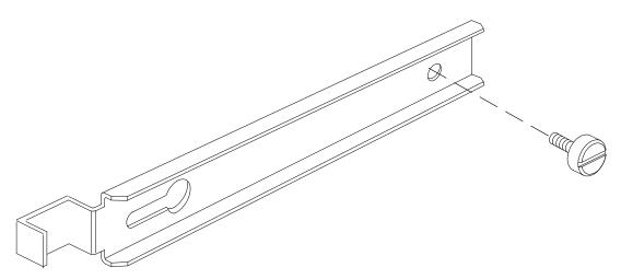
The locking bar must be installed on both the front and the rear of the units, in the positions shown in the following figure.
