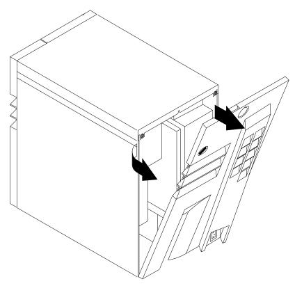
4. Pull the cover upward, to remove it from the cabinet.
