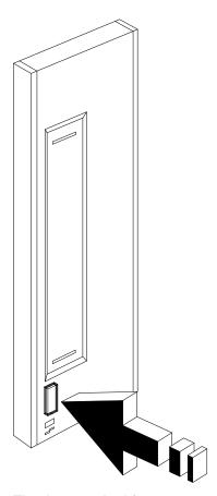
The time required for a tape to rewind and unload is between 18 seconds and 3 minutes, depending on the position of the tape when the unload button is pushed.
