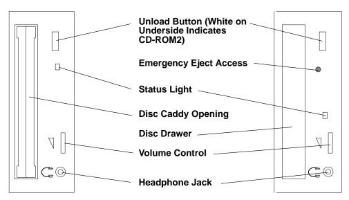
The Type B Bezel front panel has an unload button, status light, volume control, headphone jack, and disc caddy opening.
