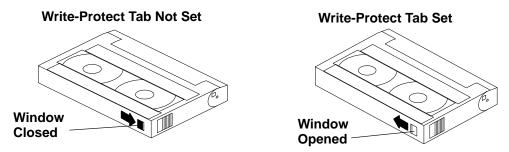
**Note:** The write-protect setting for the 4 mm tape is the opposite of the setting for the 8 mm tape.
