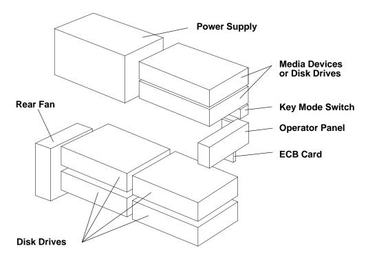
From the left side of the disk expansion unit, the following modules are accessible:
