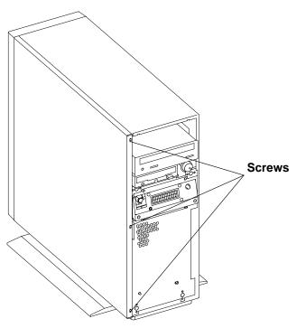
3. With a firm grip on the panel, rotate it slightly to the left while pulling it forward.
