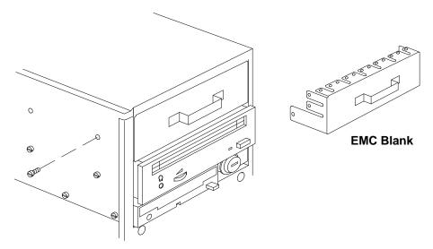
b. Install the plastic blank in the area corresponding to the empty slot. Access the front panel from its internal side and keeping the plastic blank front side facing forward, insert the left tongue of the blank in the dedicated slit on the panel. Secure the plastic blank to the panel tightening the retaining screw located on the right.
