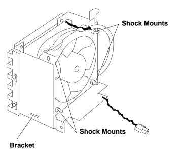
13.Lift up and remove the fan module from the bracket.
