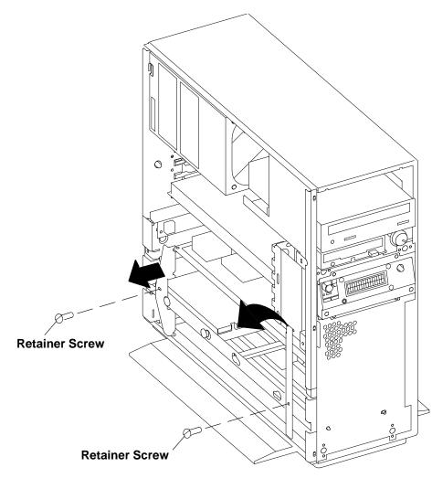
2. Slide the upper tongue of the CPU/memory cards retainer out of the slit located on the front fan support.
