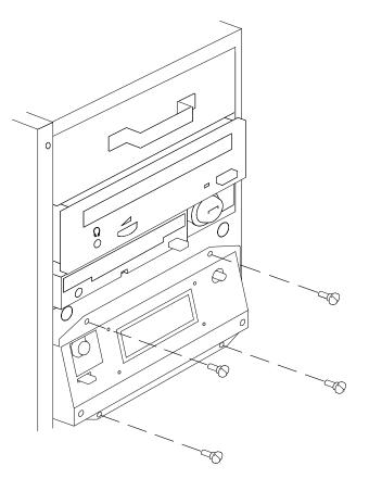
3. Move the operator panel from left to right to help remove it from its slot.
