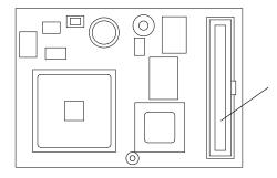
Connector used to place the KBD card on the system planar
