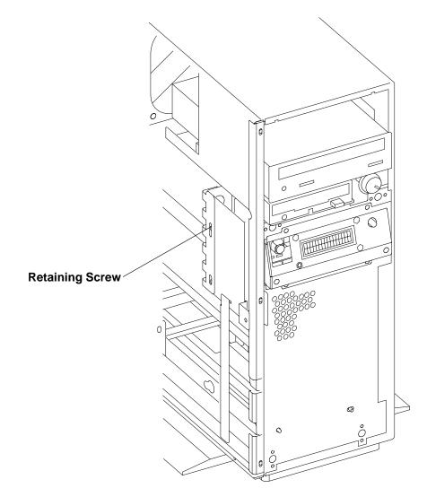
8. On the front fan cage, loosen the retainer screw which locks the adapters.
