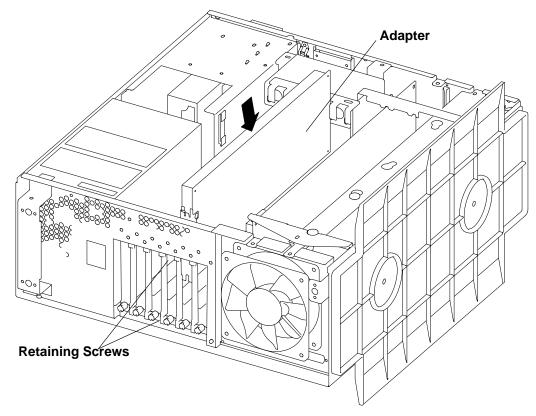
4. Secure the adapter in the slot by tightening the retaining screws on the rear side of the system unit.
