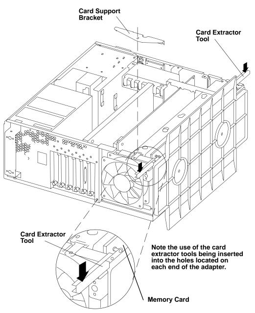
6. Slide the board out of the slot by pressing the extractors toward the system unit frame.
