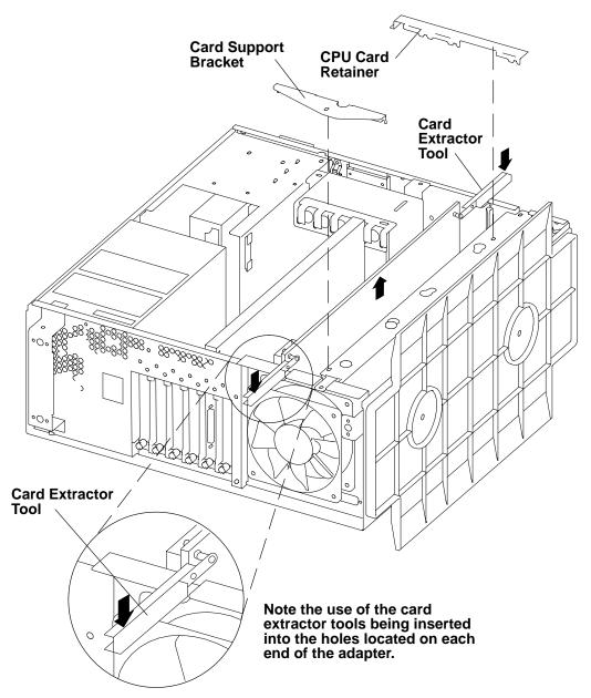
8. Slide the board out of the slot by pressing the extractors toward the system unit frame.
