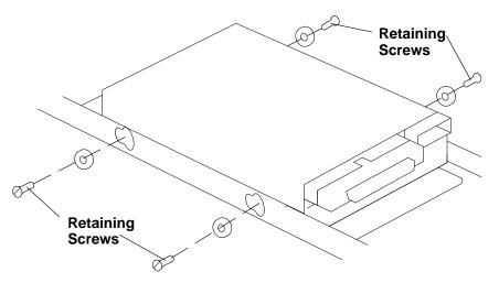
10.Lift the disk drive out of the support tray.
