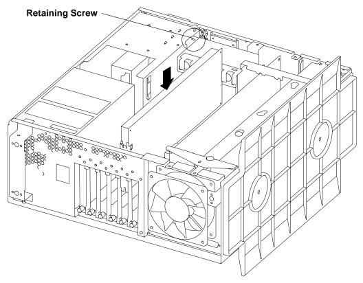
11. Lift the fan and bracket assembly from the system.
