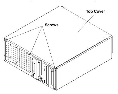
8. With a firm grip on the cover, rotate it slightly to the left while pulling the cover upward.
