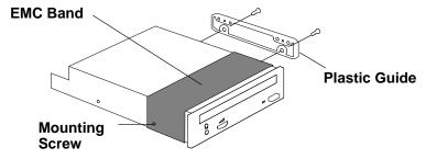
7. Remove the mounting screws for the EMC band, if installed, from the device. (The EMC band will be installed on the new device using these mounting screws.)
