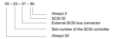
As an aid, your MediaStreamer system has several identification labels on the drawers. The drawer ID should match the slot location of the adapter that drives it. SCSI devices may be labeled with a number that identifies the SCSI address to which the device is set.
