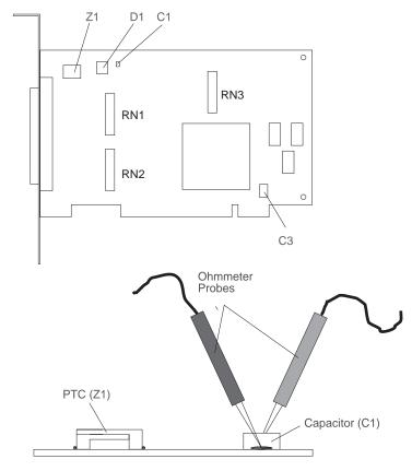
**Note:** Only the probe tips are touching the solder joints. Do not allow the probes to touch any other part of the component.
