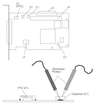
**Note:** Only the probe tips are touching the solder joints. Do not allow the probes to touch any other part of the component.
